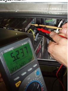
Adjust the 5V Output (labeled V1 - G1) to 5,2-5,3V.
