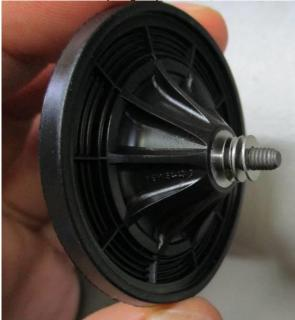
7- Screw the new diaphragm (12), complete with diaphragm spacers (13), into the connection rod (clockwise) and tighten it by hand
