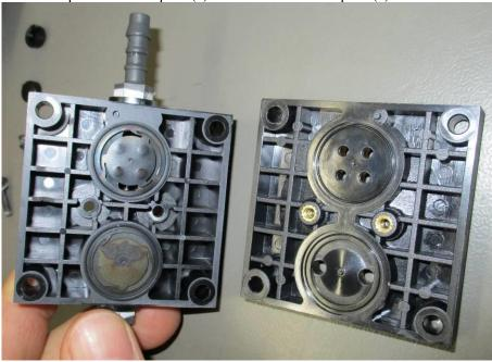
10- Remove the valve plates (2) from the intermediate plate (1). Check that the valve seats in the head plate and intermediate plate are clean
