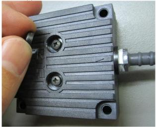
9- Separate the head plate (3) from the intermediate plate (1)
