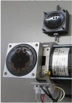
4- Turn the fan to bring the diaphragm to top dead centre. Lift the edge of the diaphragm (12) and, gripping it on opposite sides, unscrew it by turning anti-clockwise
