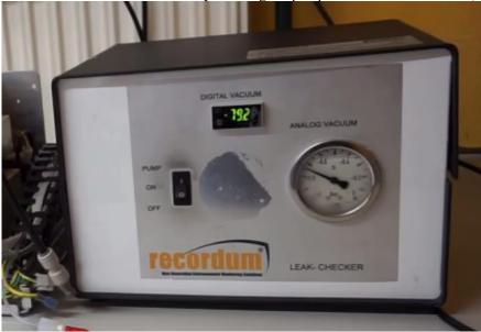
Step 3- When the pressure is stable, turn off the pump: the pressure on the manometer should stay at the same value; if it goes back to atmospheric pressure, there is a leak somewhere
