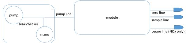
Step 2- Turn on the pump: the pressure on the manometer should go down close to 0, because the pump sucks the air and creates a vacuum: no air can enter; the pump is not strong enough to create a high vacuum, but typically below 200 mbar (200 mbar  $\approx$  -80 hPa on the digital vacuum display of the leak checking tool). The reference value can be measured by blocking the pump line of the leak checker (without any module connected).
