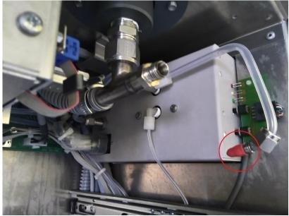
NB: The bypass circled in red in the 2 photos above is the T junction allowing the excess gas to escape through the sample fan.
