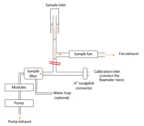
2- Compare the flowmeter reading to the total sample flow according to the following table:
