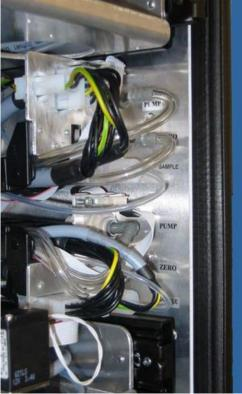
3- Disconnect the sample inlet of the desired module. Attach a flowmeter to the sample tube leading to the module. Ensure that the inlet of the flowmeter is at atmospheric pressure
