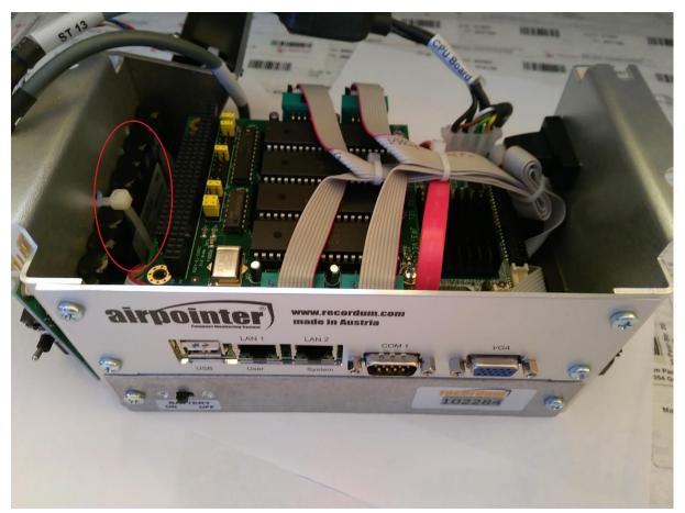
5- Screw back the lower cover of the PC, then reinstall the PC in the airpointer
