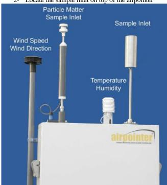
3- Unscrew the basis of the sample inlet and remove it from the airpointer
