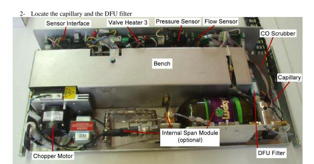
3- Unlock the push-fit connectors holding the DFU filter, remove the DFU filter, and install a new DFU filter in the same position. Then, remove the push-fit connectors holding the capillary, inspect it and if necessary, install a new capillary. In the absence of flow / pressure / leak problems, and if the capillary looks clean and intact, put the capillary back in place
