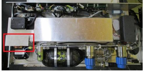
3- Unscrew the 4 screws holding the cover of the IR source and remove the cover
