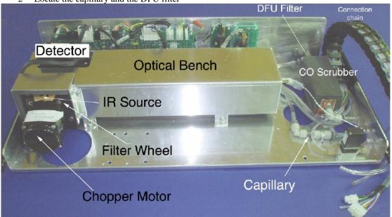
3- Unlock the push-fit connectors holding the DFU filter, remove the DFU filter, and install a new DFU filter in the same position. Then, remove the push-fit connectors holding the capillary, inspect it and if necessary, install a new capillary. In the absence of flow / pressure / leak problems, and if the capillary looks clean and intact, put the capillary back in place.
