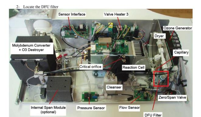
3- Unlock the push-fit connectors holding the DFU filter, remove the DFU filter, and install a new DFU filter in the same position
