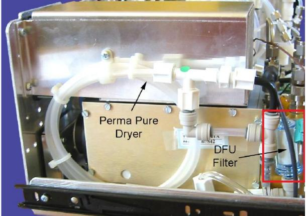
3- Unlock the push-fit connectors holding the DFU filter, remove the DFU filter, and install a new DFU filter in the same position
