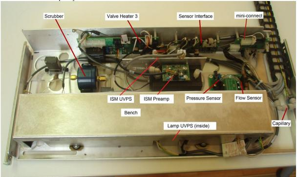
3- Remove the push-fit connectors holding the capillary, inspect it and if necessary, install a new capillary. In the absence of flow / pressure / leak problems, and if the capillary looks clean and intact, put the capillary back in place
