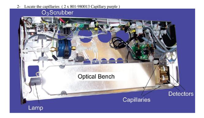
3- Remove the connectors holding the capillary, inspect it and if necessary, install a new capillary. In the absence of flow / pressure / leak problems, and if the capillary looks clean and intact, put the capillary back in place
