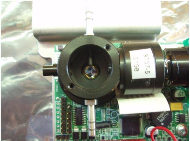
9- Screw back the lid to the chamber and reconnect the multiPM to the airpointer by following steps 1 to 4 in the reverse order
