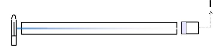
If the sample contains ozone, some of the light will be absorbed. The output of the detector then corresponds to "I" in the Lambert-Beer equation.
