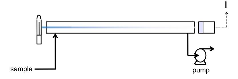
If the sample contains ozone, some of the light will be absorbed. The output of the detector then corresponds to "I" in the Lambert-Beer equation.
