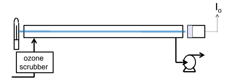
At the ozone scrubber, all ozone is destroyed. No other influence on the measuring gas occurs. The output of the detector is the  $I_0$  in the Lambert-Beer equation:
