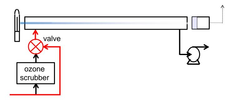
In our module the valve switches every six seconds. This enables us nearly continuous measurements of the ozone concentration.
