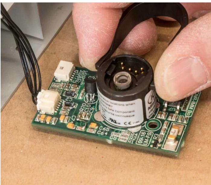
7- Carefully remove the old lamp from the detector using tweezers
