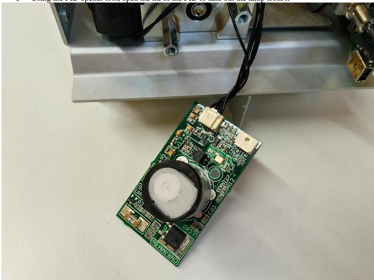
6- Using the PID opener tool, open the lid of the PID slowly, to avoid the lid from jumping out
