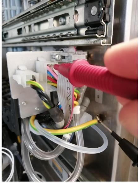
2- If any of the voltages are slightly below the nominal level, the voltage can be increased at the DC power supply (cf. paragraph 1). If there is a difference of over 0.5V between the values measured at the power supply and at the module, it is a sign that a connector is loose, dirty, or rusty, and should be therefore be cleaned or replaced.
