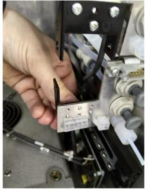
4- Remove the black heat-shrink tube, taking care of not cutting the wires below
