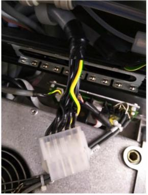
8- Spray a small amount of contact cleaning spray on the male connector. Plug it into and unplug it from the female connector a few times to have the spray evenly distributed around the pins. Let it dry completely before repowering the airpointer
