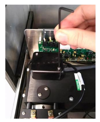
5- Disconnect the 2 cables linking the detector to the IR source
