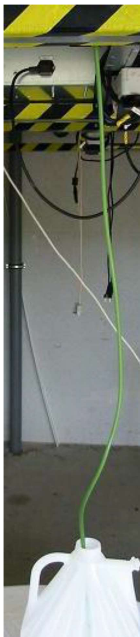
Figure 11-8: Inserting the hose into the collection container – NOT to the container bottom
