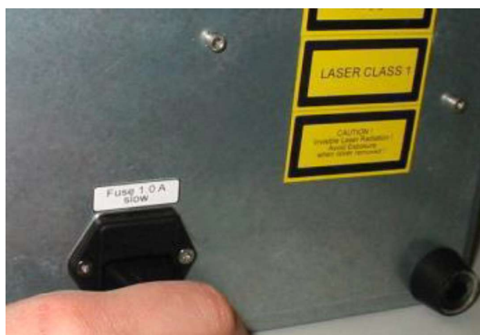
Figure 11-24: Connecting the mains cable
