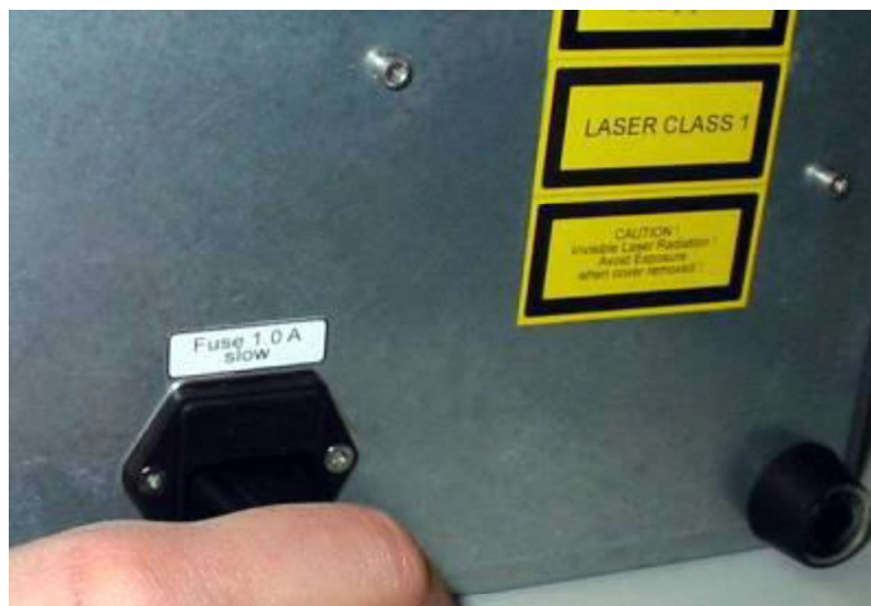
Figure 11-3: Disconnecting the device from the mains network
