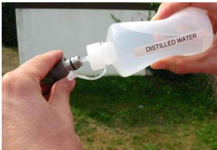
Figure 11-12: Using a bottle ② to rinse the sample collection head
