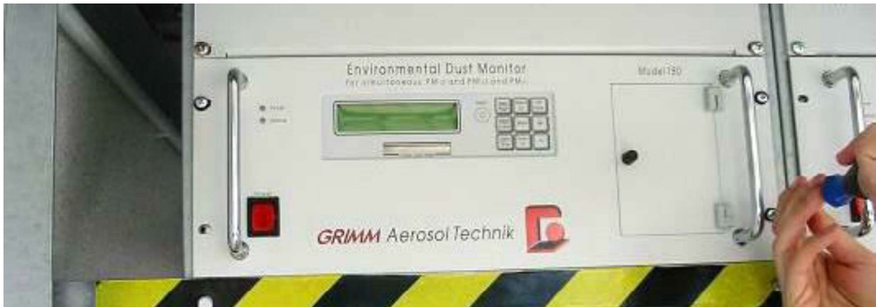
Figure 11-21: Sliding the EDM 180 into the container rack and mounting it with four screws
