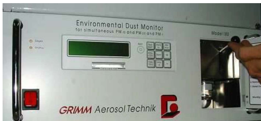
Figure 11-23: Pushing the lift lever all the way up
