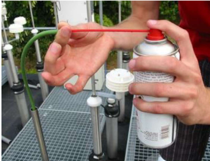
Figure 11-16: Blowing out the sample collection tube with compressed air
