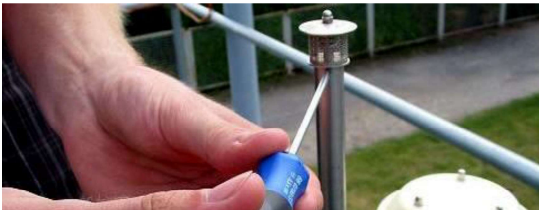
Figure 11-9: Removing the screws securing the sample collection head
