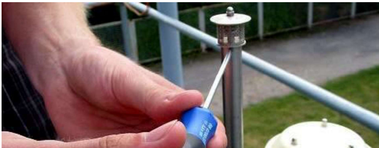
Figure 11-19: Installing the sample collection head
