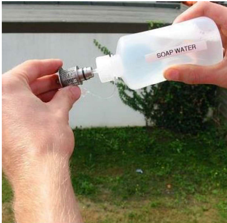
Figure 11-11: Filling the bottle ① with soap solution
