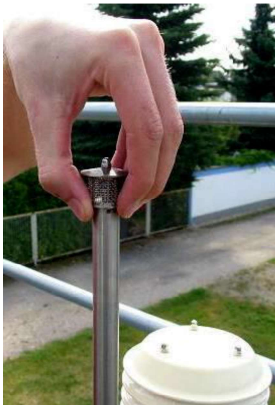
Figure 11-10: Pulling the head off the sample collection tube with a combined twisting and pushing motion
