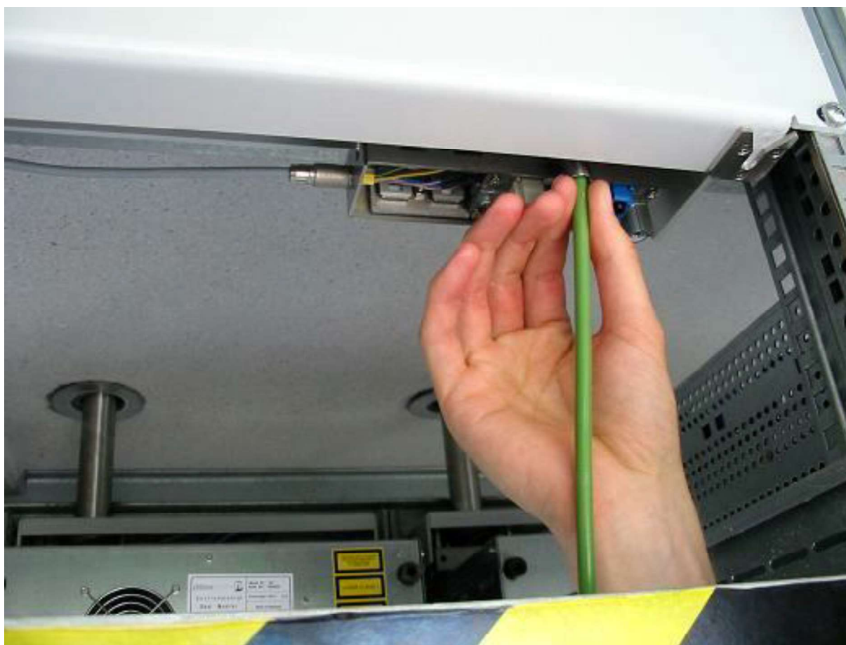
Figure 11-18: Removing the long silicone hose and collection container
