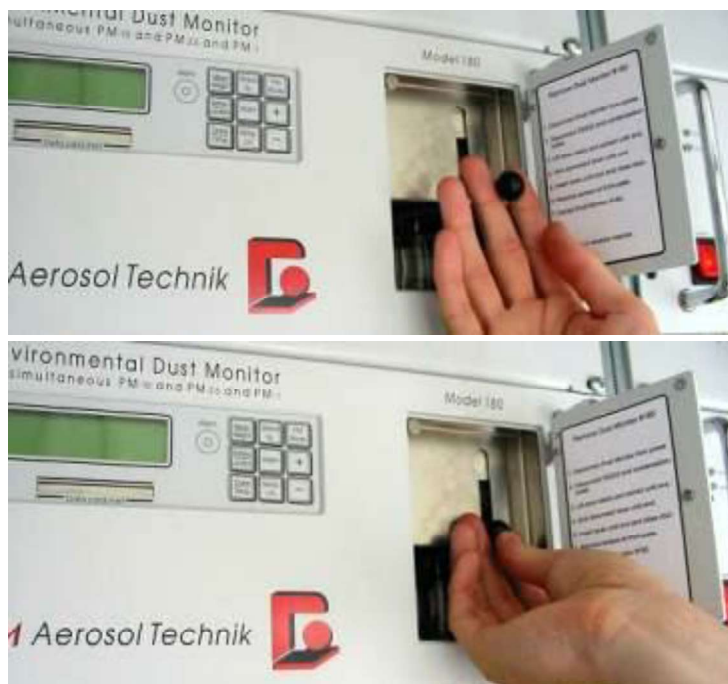
Figure 11-5: Pulling the lift lever down and sliding it in to the stop
