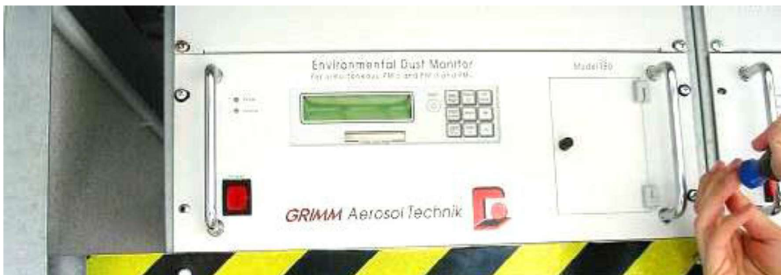
Figure 11-7: Removing the four screws from the front cover and taking the EDM 180 out of the container rack
