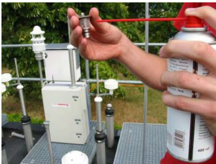
Figure 11-13: Blowing out the sample collection head with compressed air
