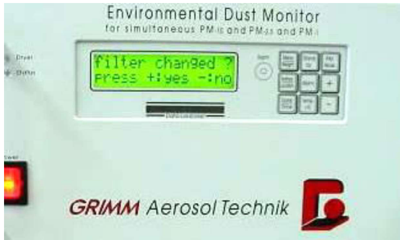
Figure 11-26: Switching on the EDM 180 and waiting for the filter query
