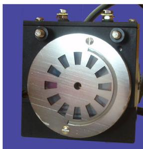
Figure 9.17.: Optical Mask for Improved S/N
