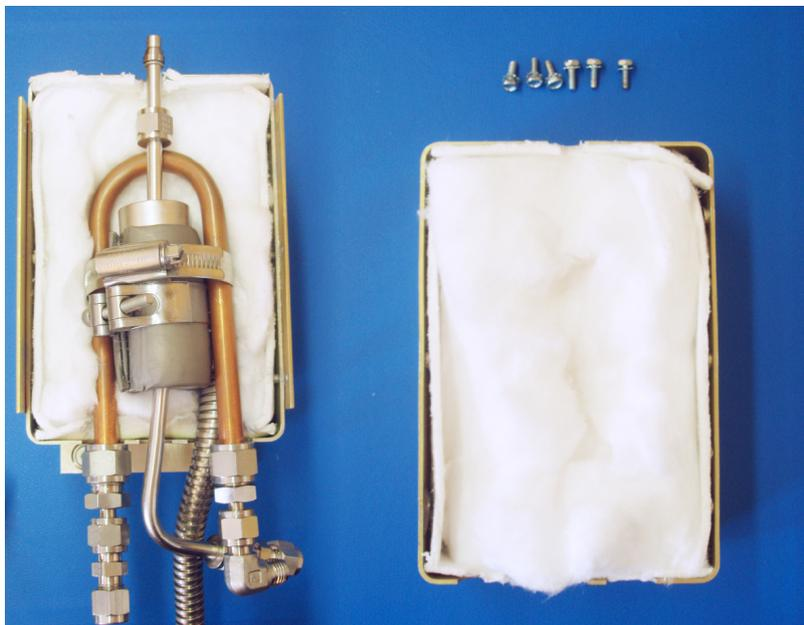
Figure 10.48.: The open Molybdenum Converter
