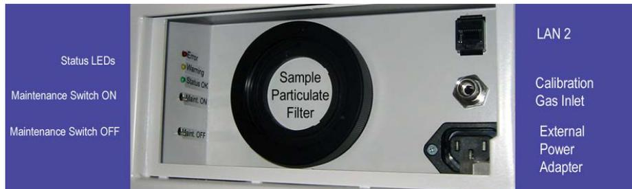
Figure 5.33.: Maintenance switches
