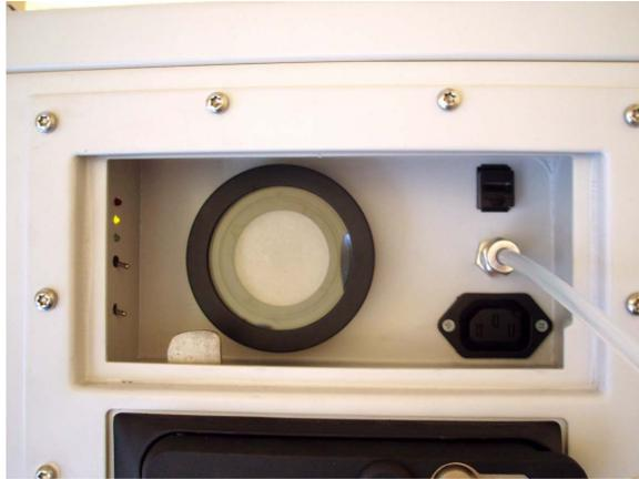
Figure 7.13.: Applying Calibration Gas to the airpointer® .
