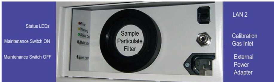
Figure 5.18.: Additional Power Socket and Status Diodes below the maintenance door
