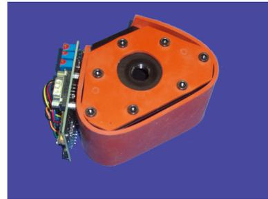
Figure 13.10.: Exterior View of a Nephelometer
