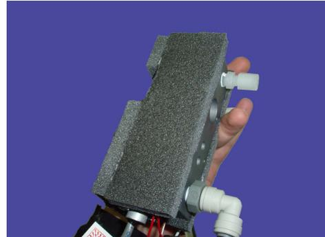
Figure 11.8.: Dismounted internal span modul with thermal insulation
