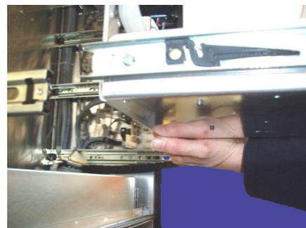
Figure 10.12.: Hold the module with one arm near the drawers
