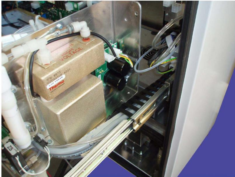
Figure 10.6.: Push and pull the module on both sides simultaneously
