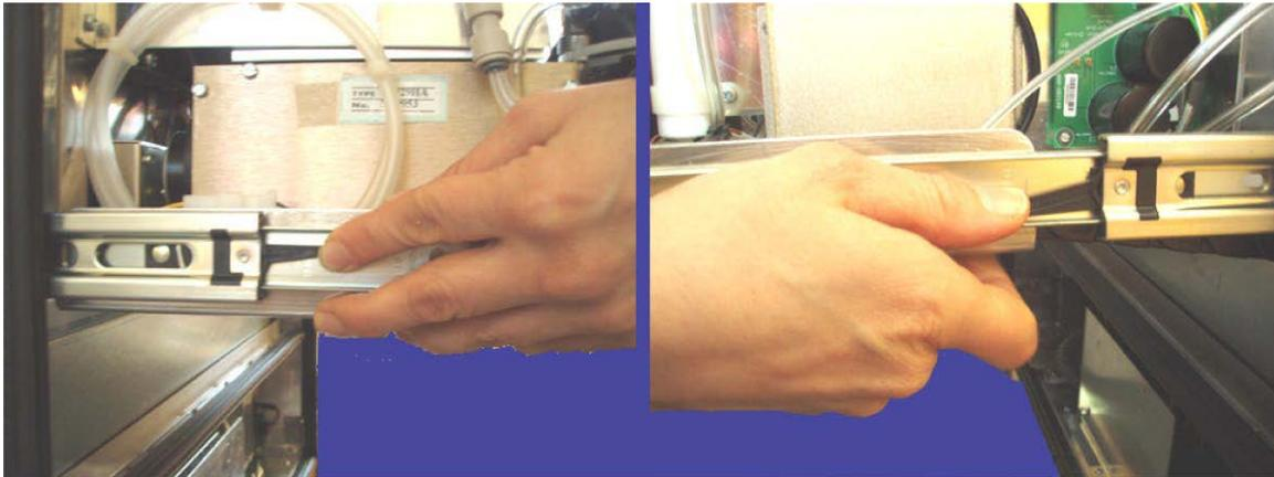
Figure 10.10.: Press the small levers in both drawers up (left) or down (right).
