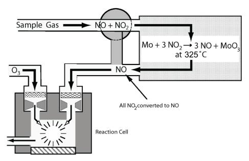
Figure 10.10.: NO<sub>2</sub> Conversion Principle
