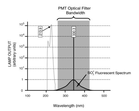
Figure 10.20.: PMT Optical Filter Bandwidth
