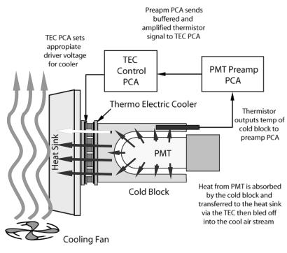
Figure 10.38.: PMT Cooling System
