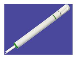
Figure 13.24.: Sensor w/o radiation shield
