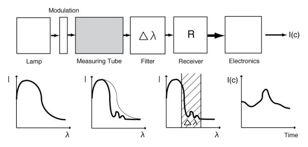
Figure 9.4.: Principle of Optical Light Detection
