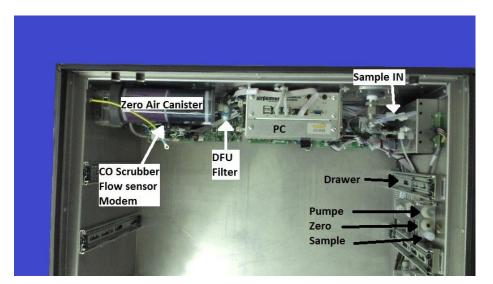
Figure 11.14.: System Components
