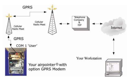
Figure 6.3.: GPRS Connection
