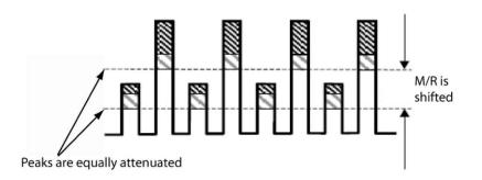
Figure 10.32.: Effects of Interfering Gas on CO MEAS and CO REF
