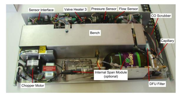
Figure 11.27.: Complete CO Module
