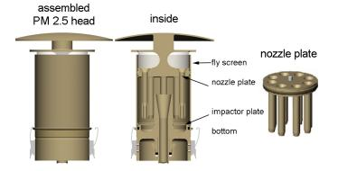
Figure 14.18.: Exterior and Interior View of the PM2.5 Head
