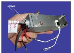
Figure 12.10.: Dismounted Internal Span Module without thermal insulation
