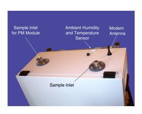
Figure 5.8.: Housing with Roof Passage
