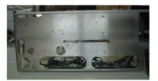
Figure 11.24.: Bottom of  $O_3$  Bench. Loosen the screws to open the bench.
