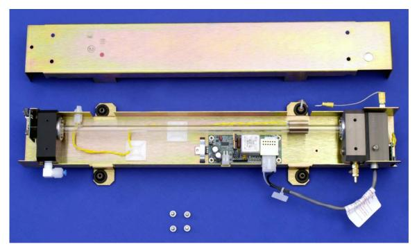
Figure 11.25.: Ozone Bench with Cover Removed
