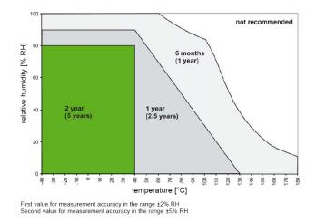
Figure 13.33.: Recalibration Interval for Humidity Sensor
