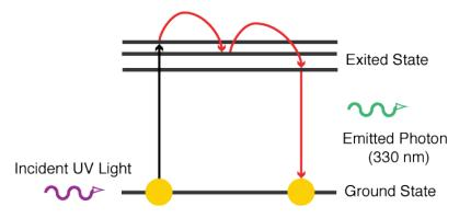
Figure 9.3.: An Excited Molecule Emits its Energy as a Light Pulse – Fluorescence.
