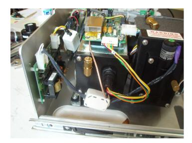
Figure 11.31.: Location of the UV Lamp Power Connector
