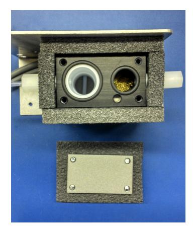
Figure 12.25.: Internal Span Module with unscrewed top and thermal insulation
