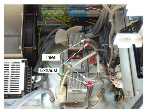
Figure 11.20.: Picture of the double piston pump from the top
