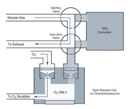
Figure 10.11.: Reaction Cell During the Auto Zero Cycle
