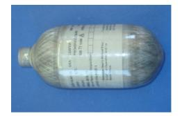
Figure 12.16.: Gas cylinder of the CO-module
