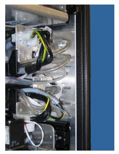
Figure 11.46.: Connection of the Flow Channel of a Module to the airpointer®
