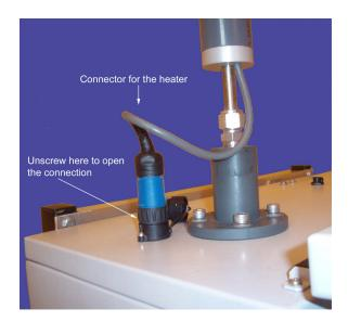
Figure 14.3.: Connect and Disconnect the Plug
