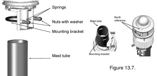
Figure 13.6.: Lufft Sensor: Mounting and North Alignment
