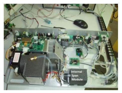
Figure 12.17.: Location of the Internal Span Module of the SO<sub>2</sub> module
