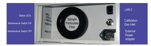
Figure 5.33.: Maintenance switches
