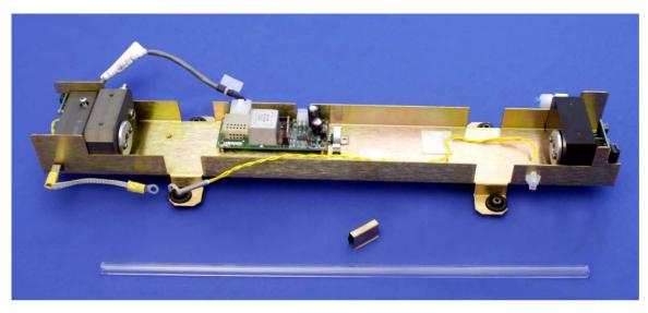
Figure 11.26.: Ozone Bench Disassembled
