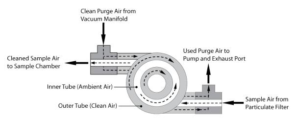
Figure 10.39.: Hydrocarbon Scrubber Scheme
