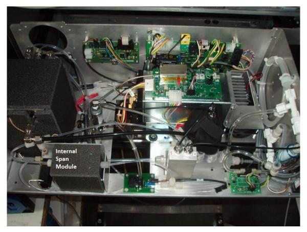
Figure 12.22.: Location of the Internal Span Module of the NO<sub>x</sub> module
