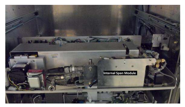
Figure 12.14.: Location of the Internal Span Module on the CO module
