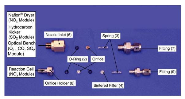
Figure 11.44.: Critical Flow Orifice Assemblies
