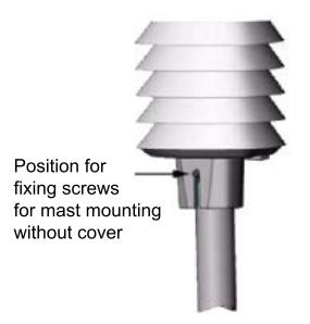
Figure 13.5.: Fixing Screws of the Vaisala Sensor
