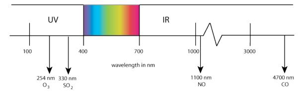
Figure 9.1.: Overview of Emitted or Absorbed Wavelengths of Measured Pollutants. The Centers of the Various Wavelength Ranges are Depicted Separately.
