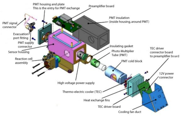
Figure 10.37.: Sensor Assembly
