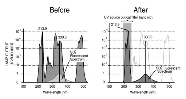
Figure 10.19.: Excitation Lamp UV Spectrum Before/After Filtration
