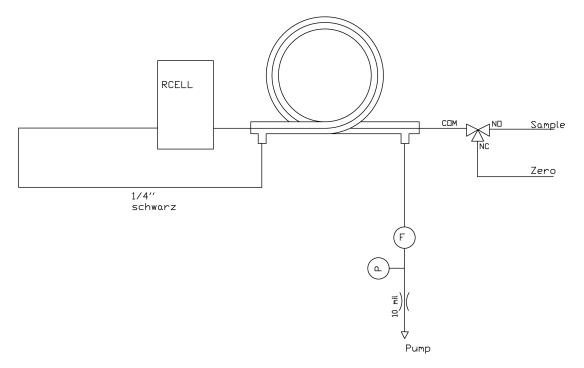
Figure 10.6.: Flow Diagram of SO<sub>2</sub> Module
