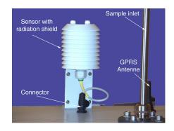
Figure 13.28.: Front view of the mounted sensor
