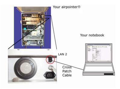
Figure 6.1.: Direct Connection
