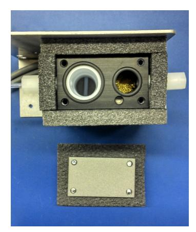
Figure 12.20.: Internal Span Module with unscrewed top and thermal insulation
