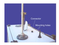
Figure 13.29.: The Sensor is Mounted in Upright Position.
