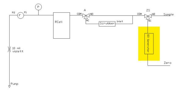
Figure 12.9.: Flow diagram of the ozone module with Internal Span Module
