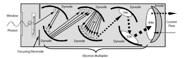
Figure 10.36.: Scheme of a Photomultiplier Tube
