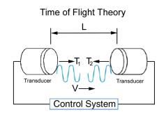
Figure 13.19.: Gill Sensor - Principle of Operation
