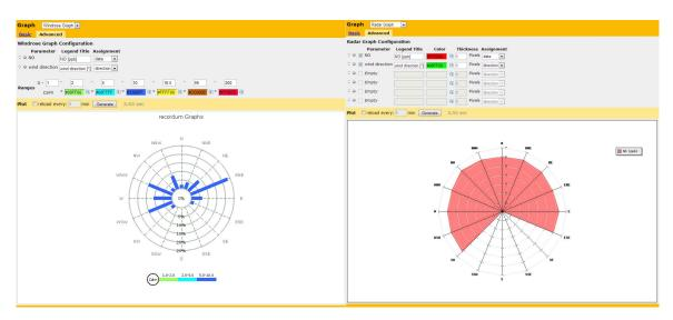
Figure 7.4.: Comparative plot of a NO measurement versus the wind direction shown in a Wind Rose (a) and a Radar Graph (b).
