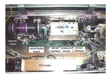
Figure 14.6.: Built-in Nephelometer
