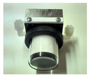
Figure 5.14.: The basic Extended Liftime Filter
