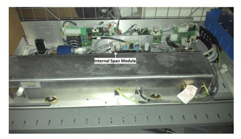
Figure 12.6.: Location of the Internal Span Module in the ozone module
