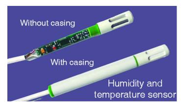
Figure 13.26.: Interior view of the sensor
