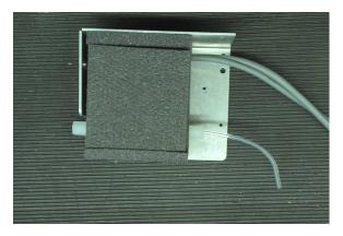
Figure 12.24.: Removed Internal Span Module with thermal insulation
