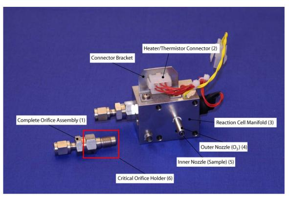
Figure 11.39.: Reaction Cell Manifold
