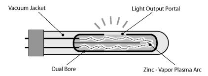
Figure 10.17.: UV Source Lamp Schematic
