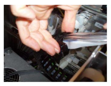
Figure 11.10.: Loose the clamp
