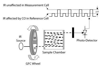
Figure 10.30.: Measurement Fundamentals Using a GFC Wheel
