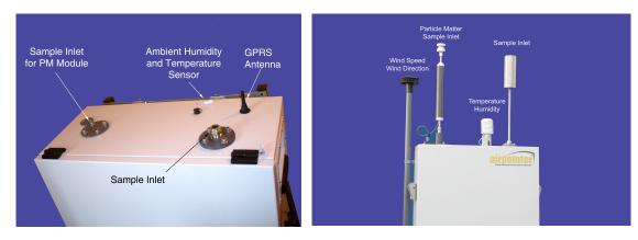
Figure 14.4.: Top View of the Hous- Figure 14.5.: Top View of the Housing without Sensors ing with Sensors (On the and Inlets left side: Sample Inlet of the PM Module with PM10 Sampling Head)
