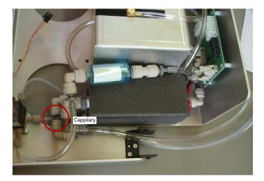
Figure 11.28.: Location of the Capillary inside the CO Module
