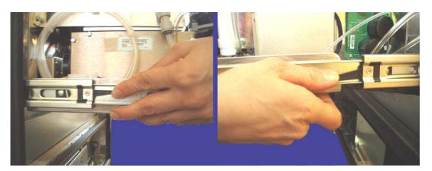
Figure 11.11.: Press the small levers in both drawers up (left) or down (right).
