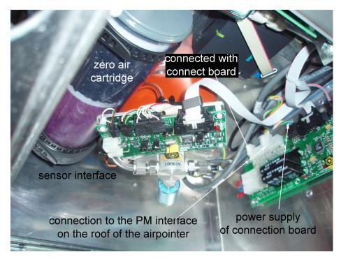
Figure 14.8.: Wiring of the Nephelometer
