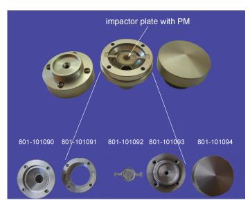
Figure 14.17.: PM10 Head Disassembled
