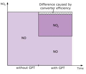
Figure 7.18.: Influence of the Converter Efficiency
