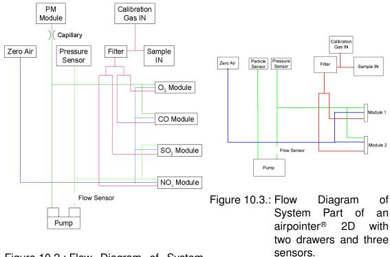
Figure 10.2.: Flow Diagram of System Part of an airpointer<sup>®</sup> 4D with four drawers and five modules.
