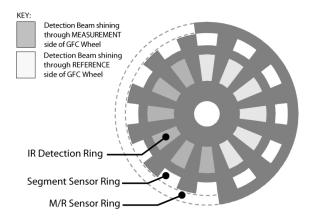
Figure 10.33.: Optical Mask for Improved S/N
