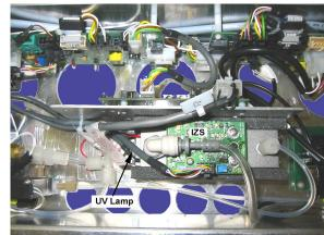
Figure 12.7.: Top view of the ozone module with installed Internal Span Module
