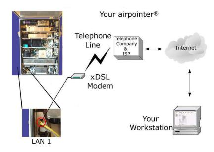
Figure 6.9.: ADSL and SDSL Connection
