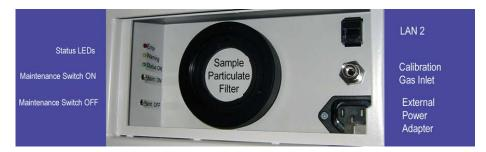
Figure 5.18.: Additional Power Socket and Status Diodes below the maintenance door
