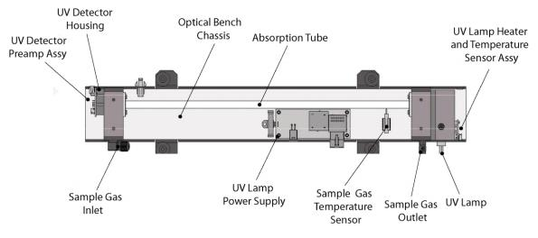
Figure 10.23.: Optical O<sub>3</sub> Bench
