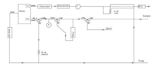
Figure 10.8.: Flow Diagram of NO<sub>x</sub> Module
