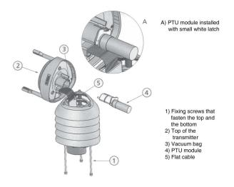
Figure 13.23.: Scheme of the open Vaisala sensor
