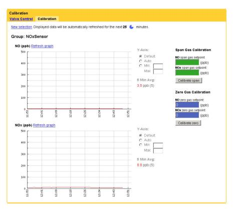
Figure 7.16.: Display of the calibration and input of the setpoints
