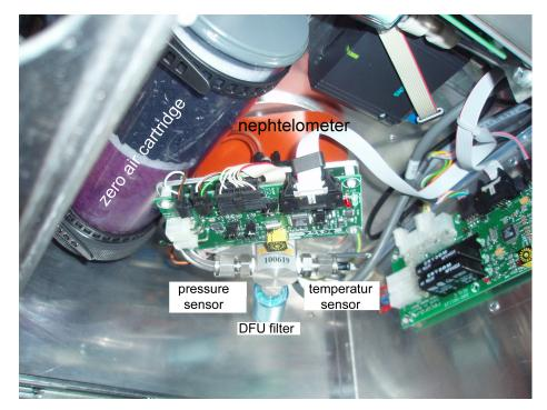
Figure 14.7.: The Position of the Nephelometer
