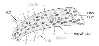
Figure 10.13.: Semi-Permeable Membrane Drying Process
