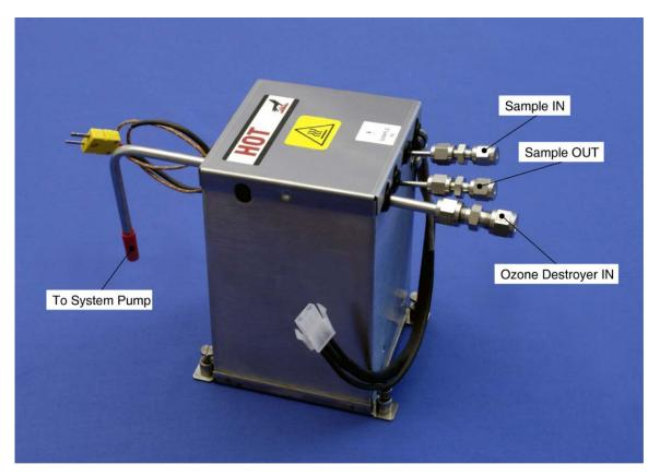
Figure 11.33.: The Molybdenum Converter Module
