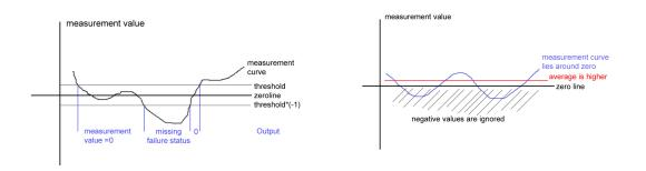
Figure 13.14.: Measurement Curve with Threshold Figure 13.15.: Measurement Curve with Suppressed Negative Values
