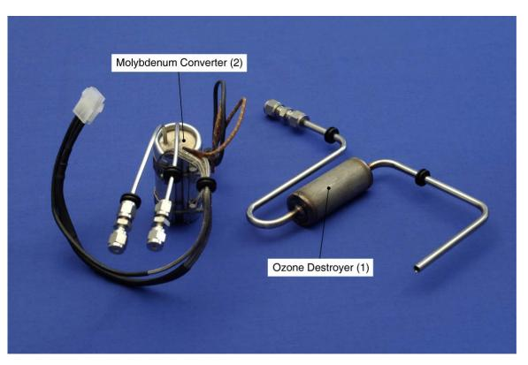
Figure 11.35.: The Converter and the Ozone Destroyer.
