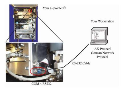
Figure 6.10.: Connection Using AK or German Ambient Network Protocol
