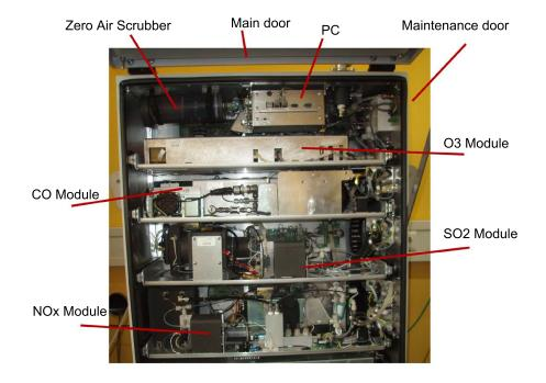
Figure 11.1.: Inside the airpointer<sup>®</sup> with four slides (4D) top
