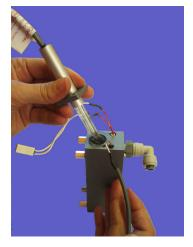
Figure 12.11.: Exchange of the UV lamp
