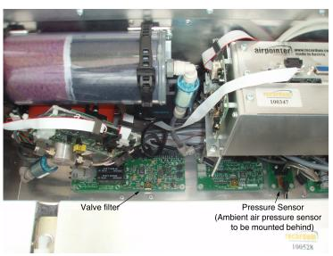
Figure 13.34.: Localization of the ambient air pressure sensor (behind the pump pressure sensor, not figured)
