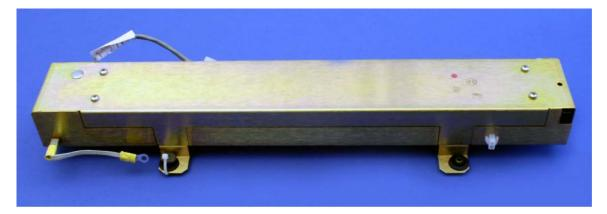
Figure 11.23.: Ozone Bench without Thermal Insulation
