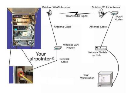
Figure 6.7.: Wireless LAN Connection
