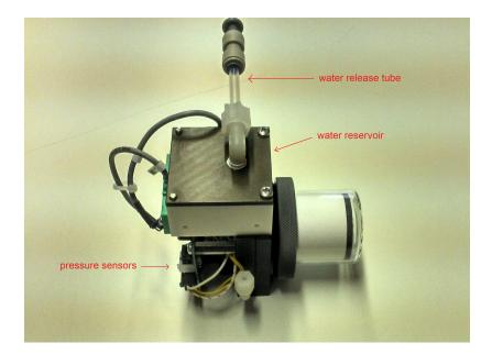
Figure 5.15.: An Extended Lifetime Filter with both options
