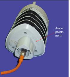
North mark on the Vaisala sensor: The arrow on the bottom of the sensor points north
