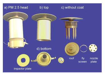
Figure 14.19.: PM2.5 Head Disassembled
