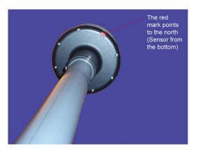
Figure 13.8.: North mark on the Gill sensor: The red point on the bottom side Figure 13.9.: North points north the v
