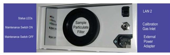
Figure 5.13.: Inside the Maintenance Door of the airpointer®
