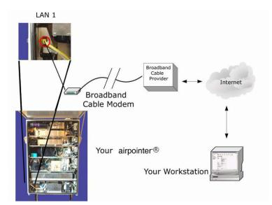
Figure 6.8.: Cable Modem Connection
