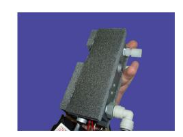
Figure 12.8.: Dismounted internal span modul with thermal insulation
