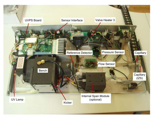
Figure 11.29.: Complete SO<sub>2</sub> Bench
