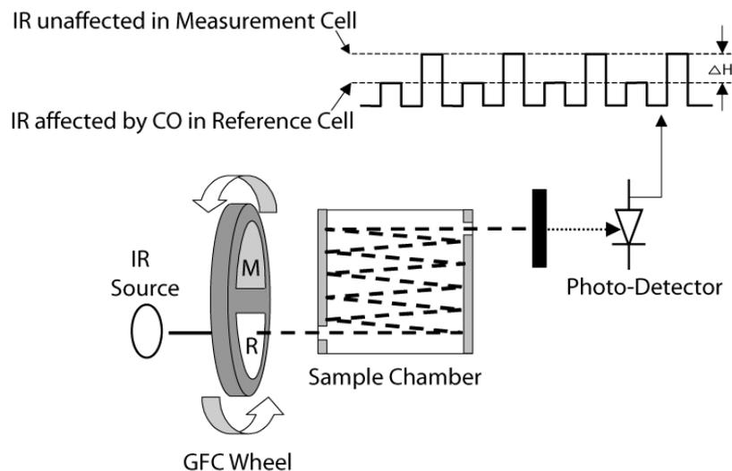
Figure 10.30.: Measurement Fundamentals Using a GFC Wheel
