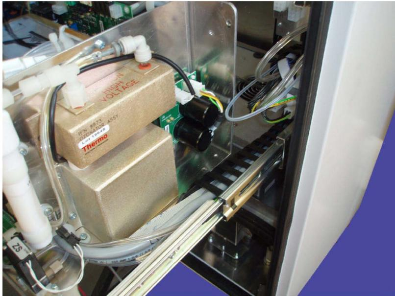
Figure 11.7.: Push and pull the module on both sides simultaneously
