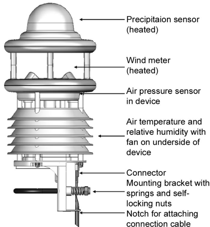
Figure 13.16.: Scheme of the Lufft Sensor WS600
