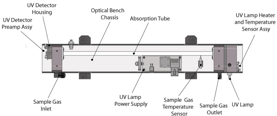
Figure 10.23.: Optical O<sub>3</sub> Bench
