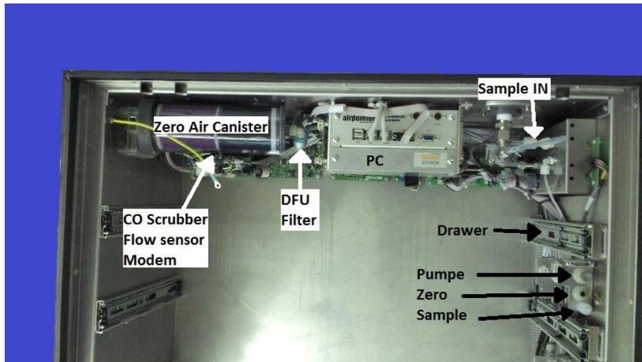
Figure 11.14.: System Components
