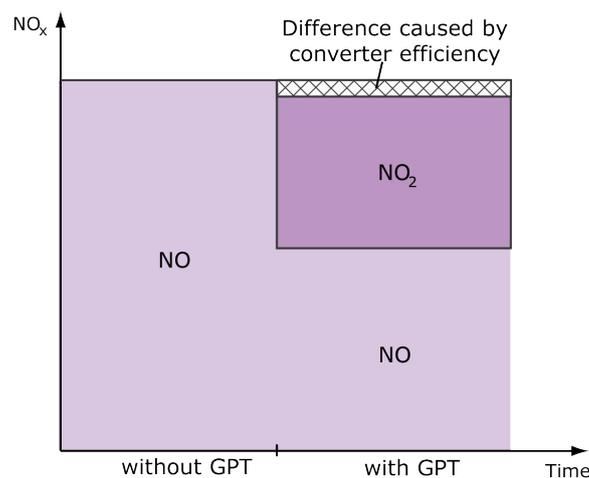
Figure 7.18.: Influence of the Converter Efficiency
