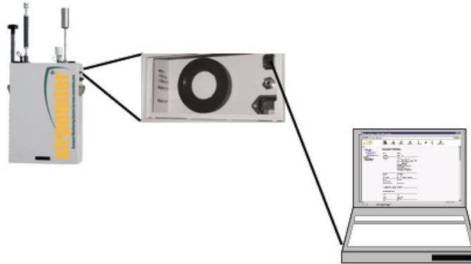
Figure 5.20.: Direct Connection
