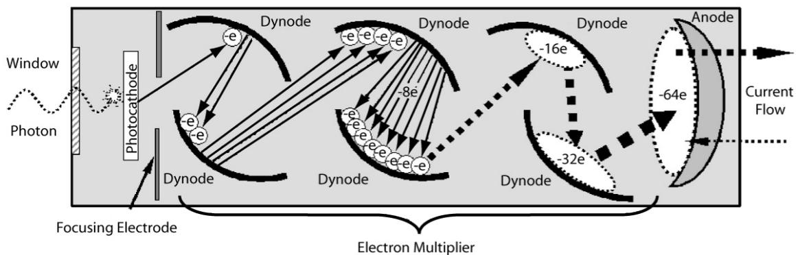
Figure 10.36.: Scheme of a Photomultiplier Tube
