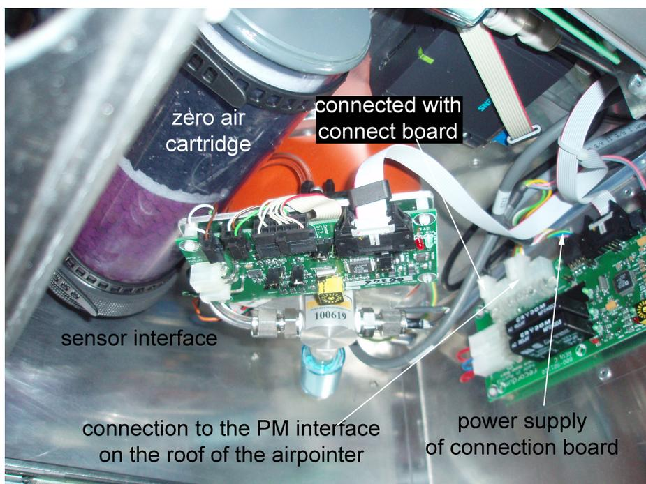
Figure 14.8.: Wiring of the Nephelometer
