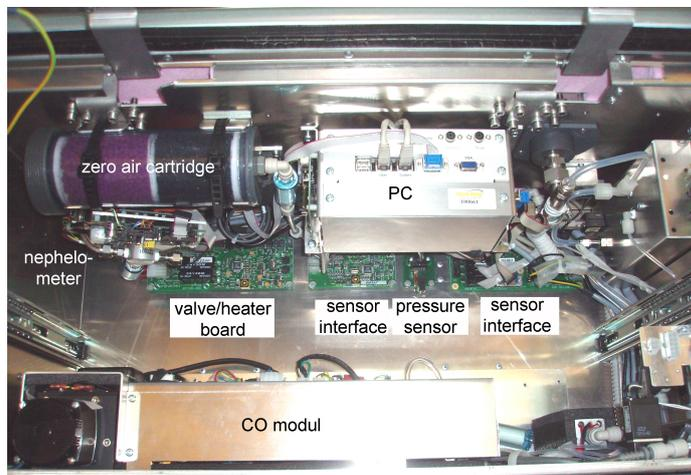
Figure 14.6.: Built-in Nephelometer
