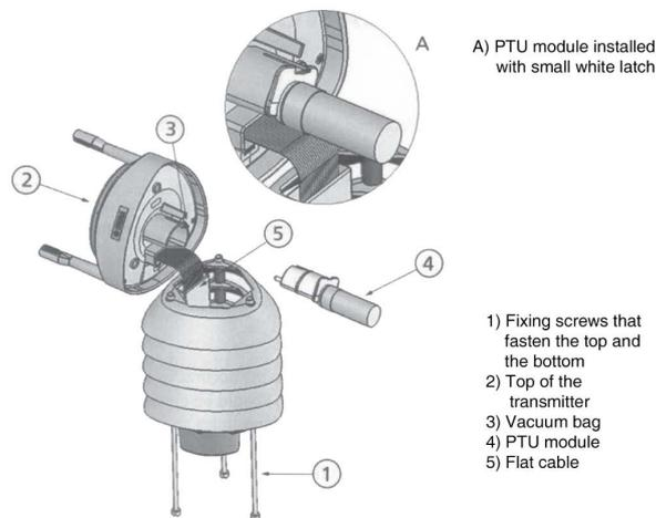
Figure 13.23.: Scheme of the open Vaisala sensor
