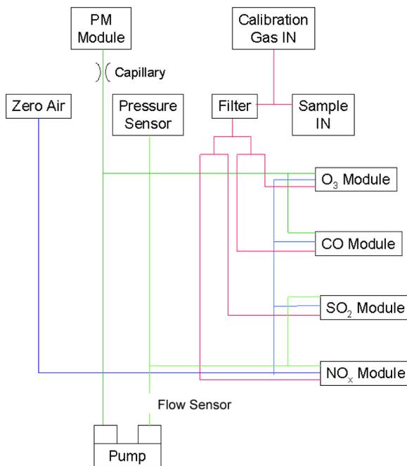
Figure 10.2.: Flow Diagram of System Part of an airpointer® 4D with four drawers and five modules.
