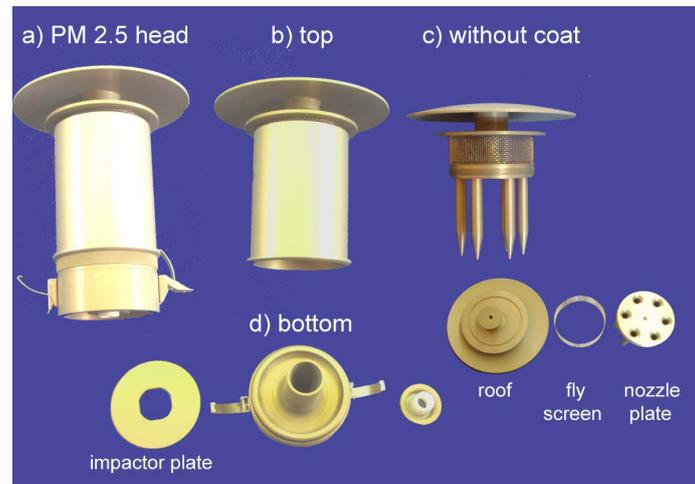
Figure 14.19.: PM2.5 Head Disassembled
