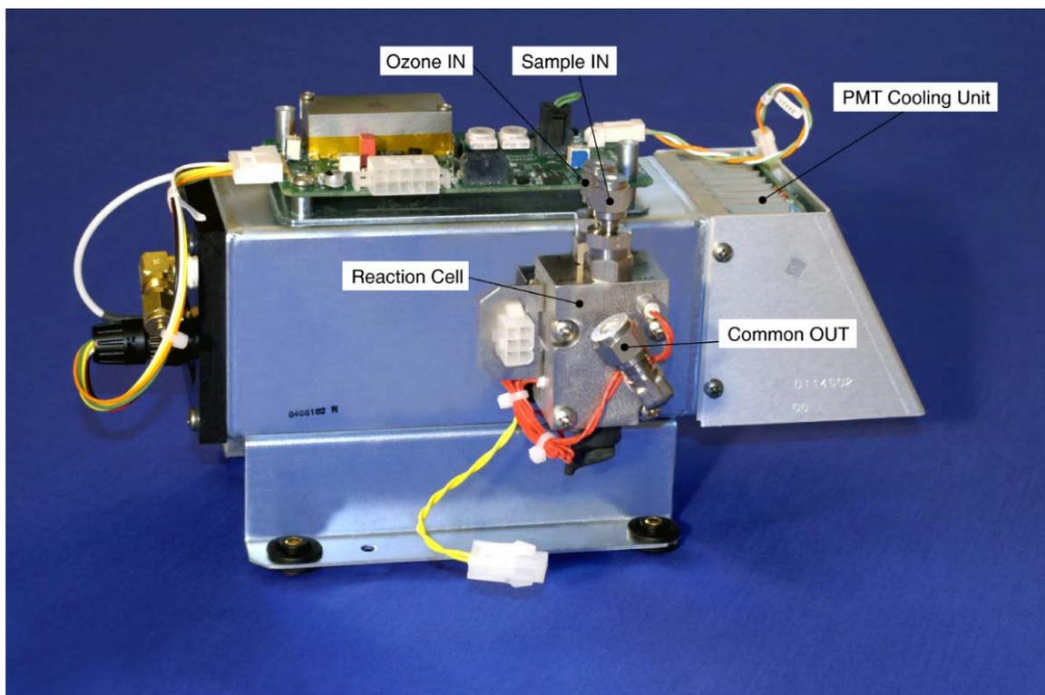
Figure 11.37.: NO<sub>x</sub> Sensor with Reaction Cell
