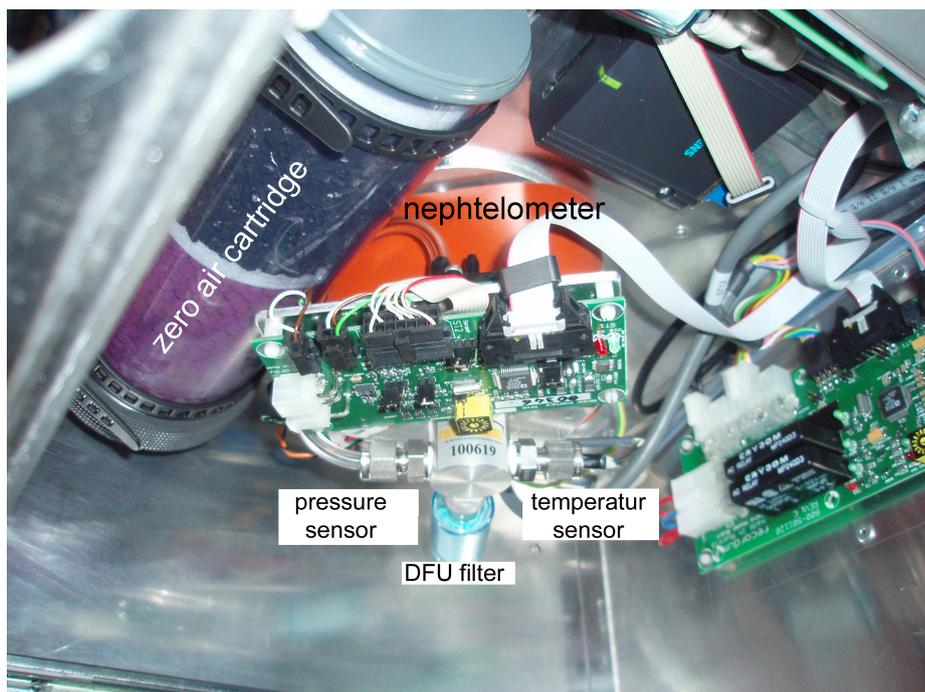
Figure 14.7.: The Position of the Nephelometer
