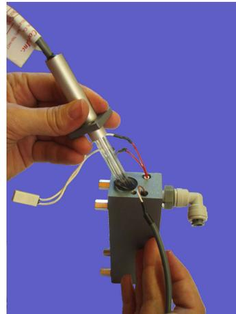
Figure 12.11.: Exchange of the UV lamp
