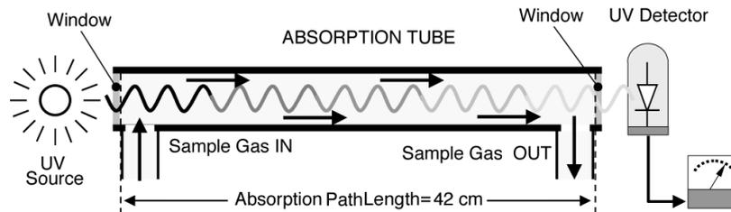
Figure 10.24.: O<sub>3</sub> Absorption Path
