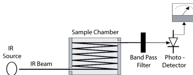
Figure 10.28.: Measurement Fundamentals
