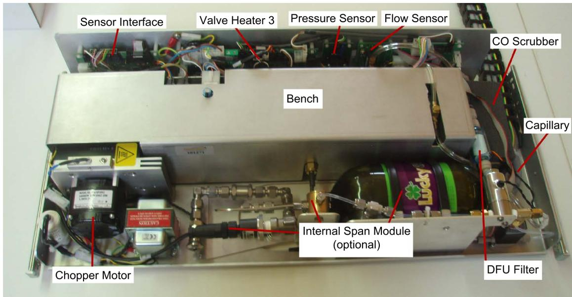
Figure 11.27.: Complete CO Module
