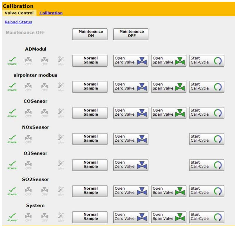
Figure 7.12.: Activate the Maintenance Mode
