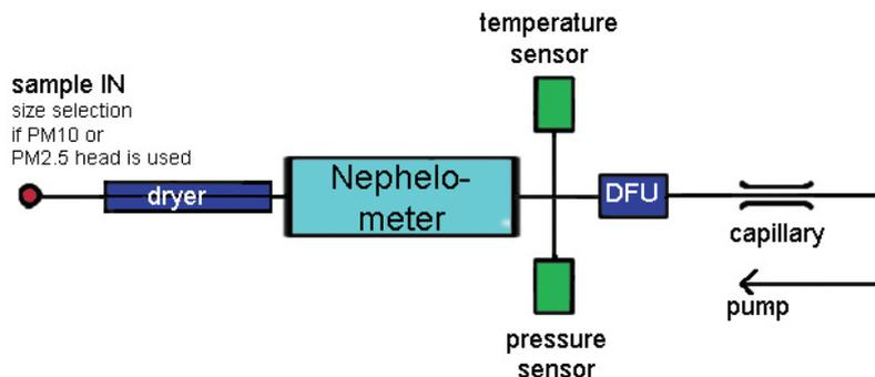
Figure 14.1.: Flow Diagram of the PM Module
