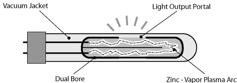
Figure 10.17.: UV Source Lamp Schematic
