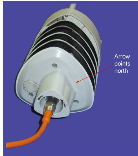
Figure 13.9.: North mark on the Vaisala sensor: The arrow on the bottom of the sensor points north
