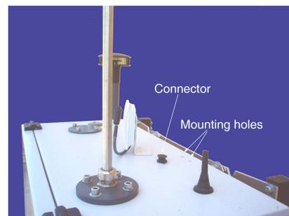
Figure 13.30.: The Sensor is Prepared for Roof Mounting.
