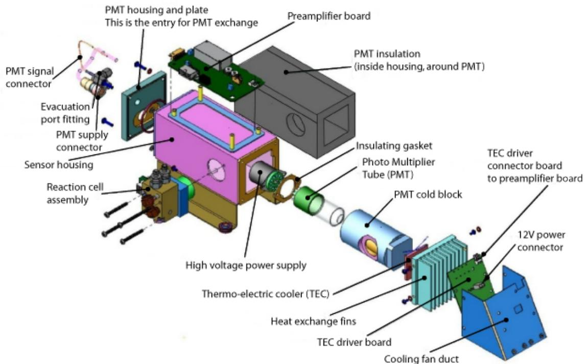
Figure 10.37.: Sensor Assembly
