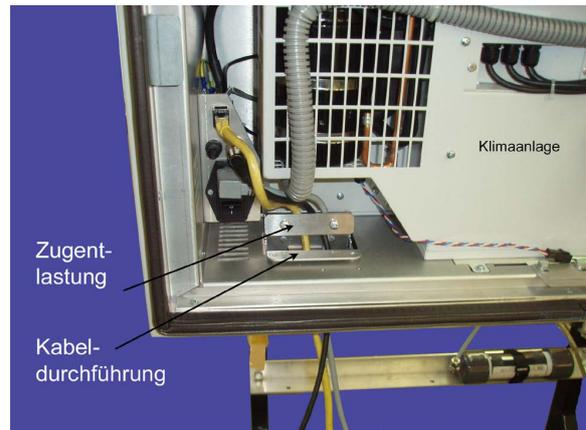
Figure 5.17.: Cable passage and strain relief
