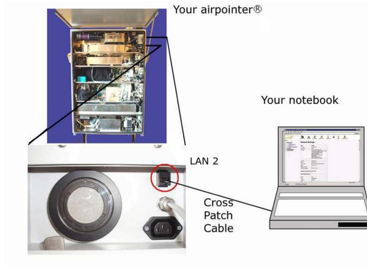
Figure 6.1.: Direct Connection
