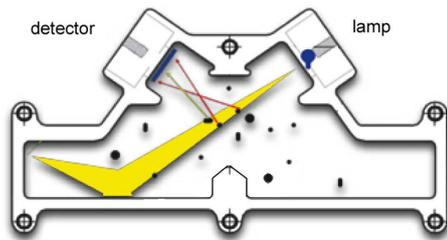
Figure 14.9.: Scheme of a Nephelometer
