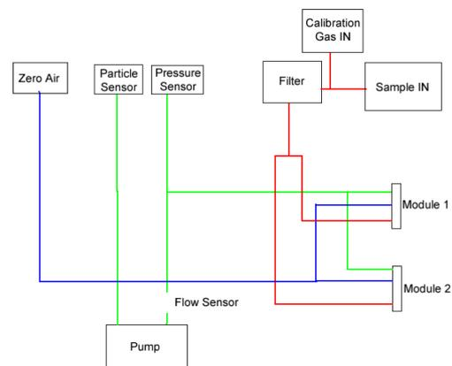
Figure 10.3.: Flow Diagram of System Part of an airpointer® 2D with two drawers and three sensors.
