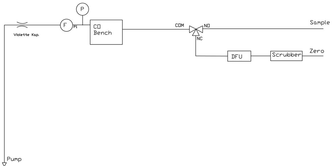
Figure 10.5.: Flow Diagram of CO Module with IZS
