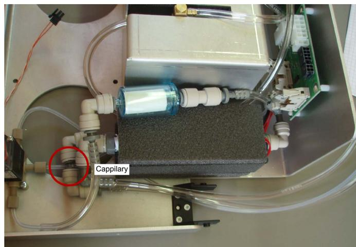
Figure 11.28.: Location of the Capillary inside the CO Module
