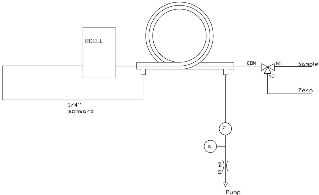
Figure 10.6.: Flow Diagram of SO<sub>2</sub> Module
