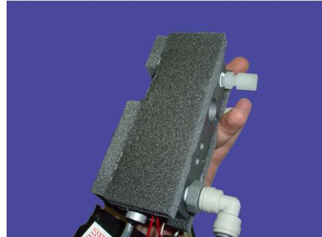
Figure 12.8.: Dismounted internal span module with thermal insulation
