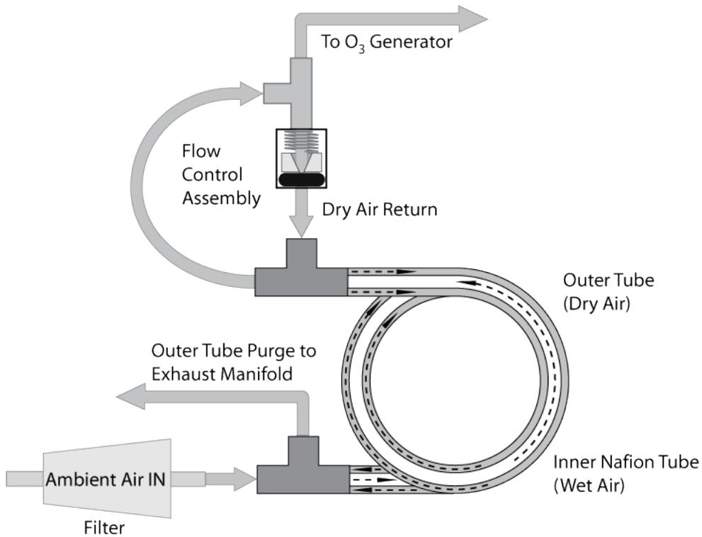
Figure 10.14.: Scheme of the Perma Pure® Dryer
