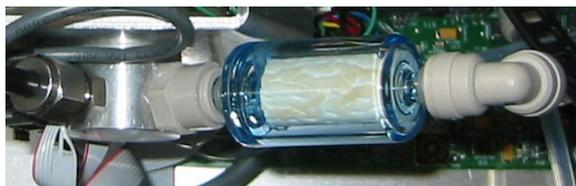
Figure 14.20.: DFU Filter at the Exit of the Nephelometer
