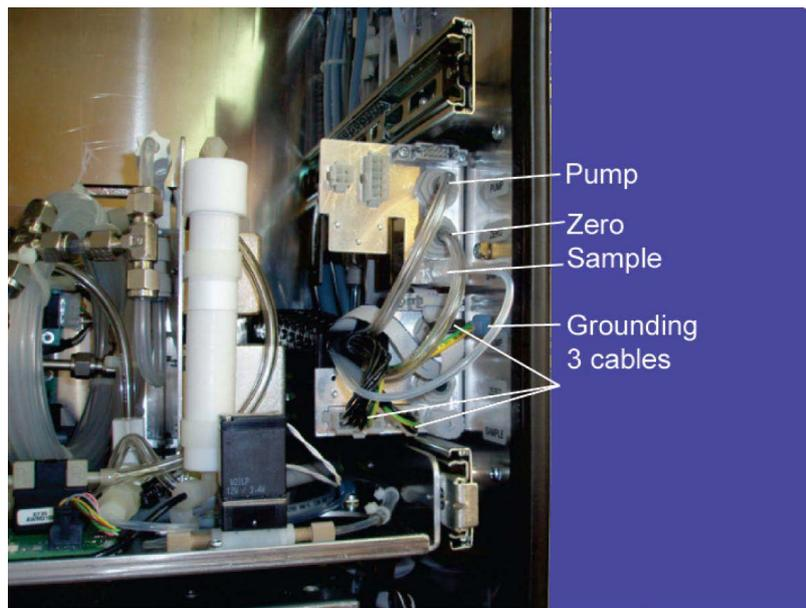
Figure 11.8.: Disconnect the seven connections of the connection chain.
