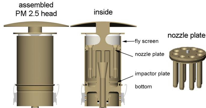
Figure 14.18.: Exterior and Interior View of the PM2.5 Head
