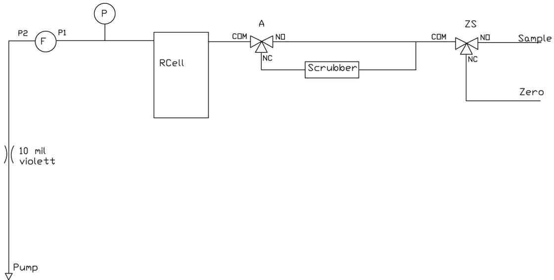
Figure 10.4.: Flow Diagram of O<sub>3</sub> Module
