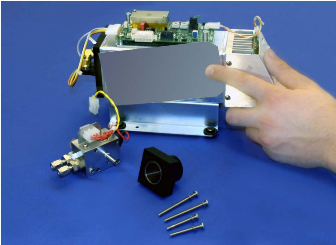
Figure 11.38.: Cover PMT Window with an Opaque Plate
