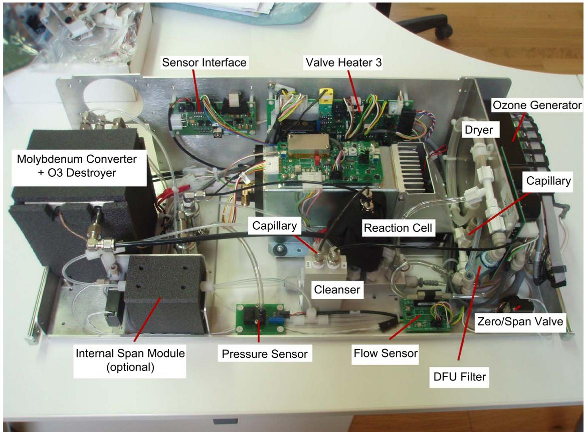
Figure 11.32.: Complete NO<sub>x</sub> Bench
