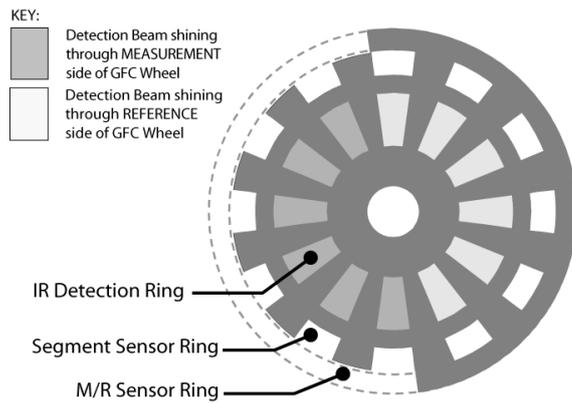
Figure 10.33.: Optical Mask for Improved S/N
