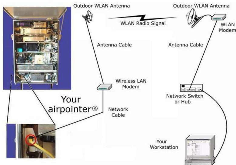
Figure 6.7.: Wireless LAN Connection
