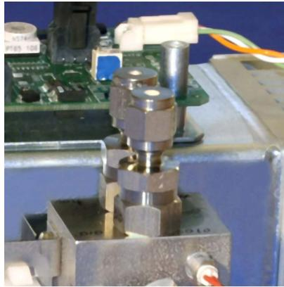
Figure 11.45.: Orifice Holders of the NO<sub>x</sub> Reaction Cell
