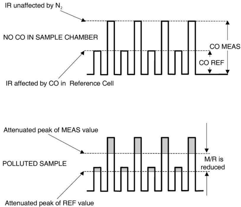
Figure 10.31.: Effect of CO in the Sample on CO MEAS and CO REF
