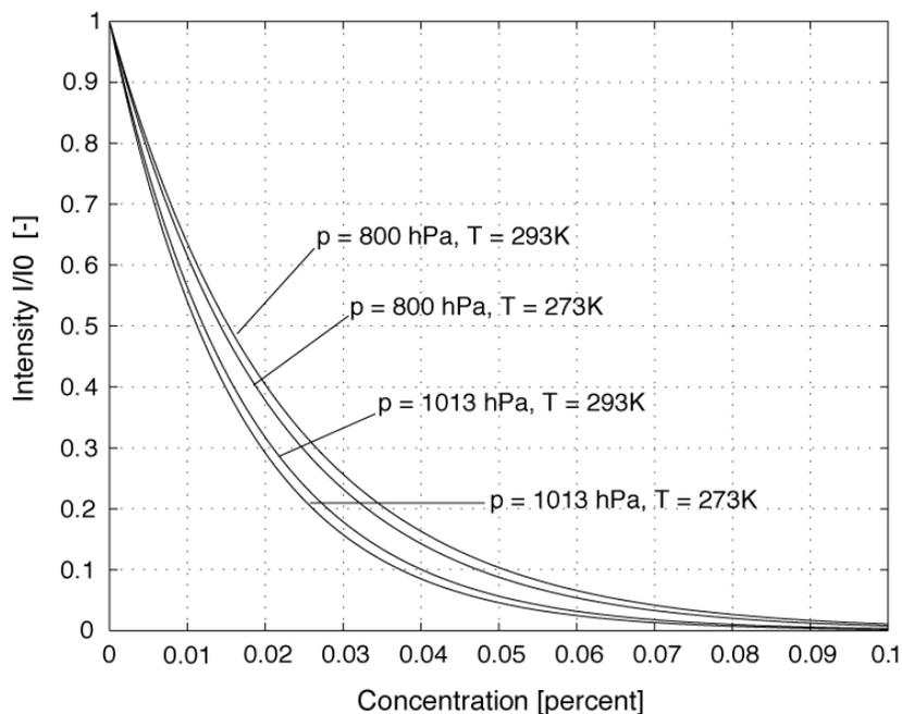
Figure 9.2.: The Law of Absorption by Lambert and Beer ( $\alpha = 308\text{m}^{-1}$ ,  $z = 0.2\text{m}$ )
