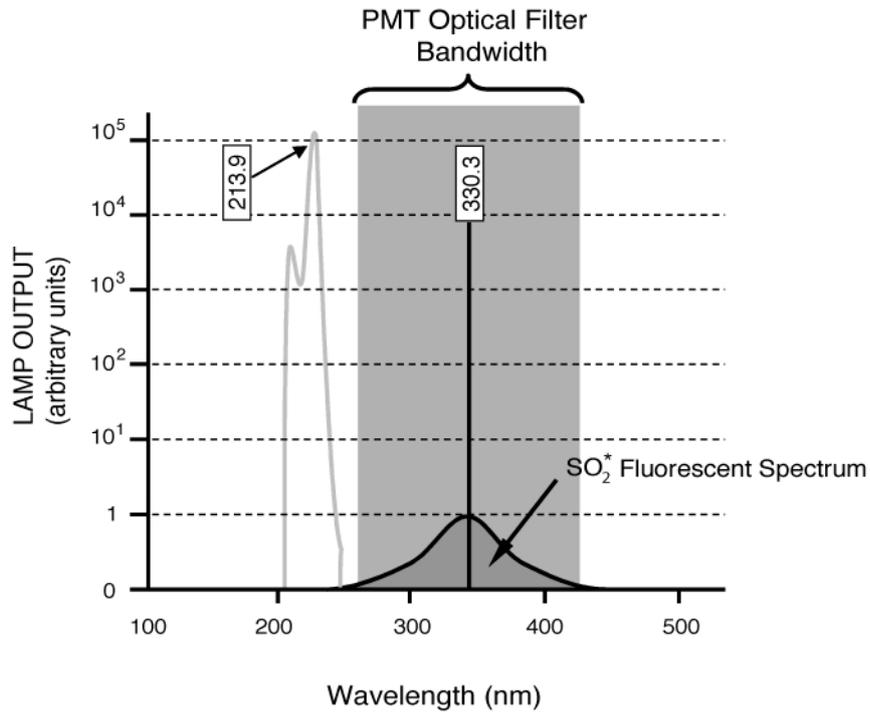
Figure 10.20.: PMT Optical Filter Bandwidth
