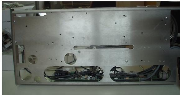
Figure 11.24.: Bottom of O<sub>3</sub> Bench. Loosen the screws to open the bench.
