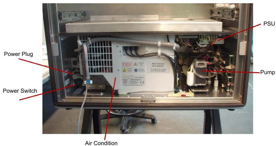
Figure 11.2.: Inside the airpointer® with four slides (4D) bottom
