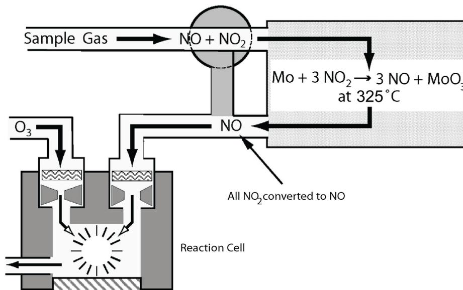
Figure 10.10.: NO<sub>2</sub> Conversion Principle
