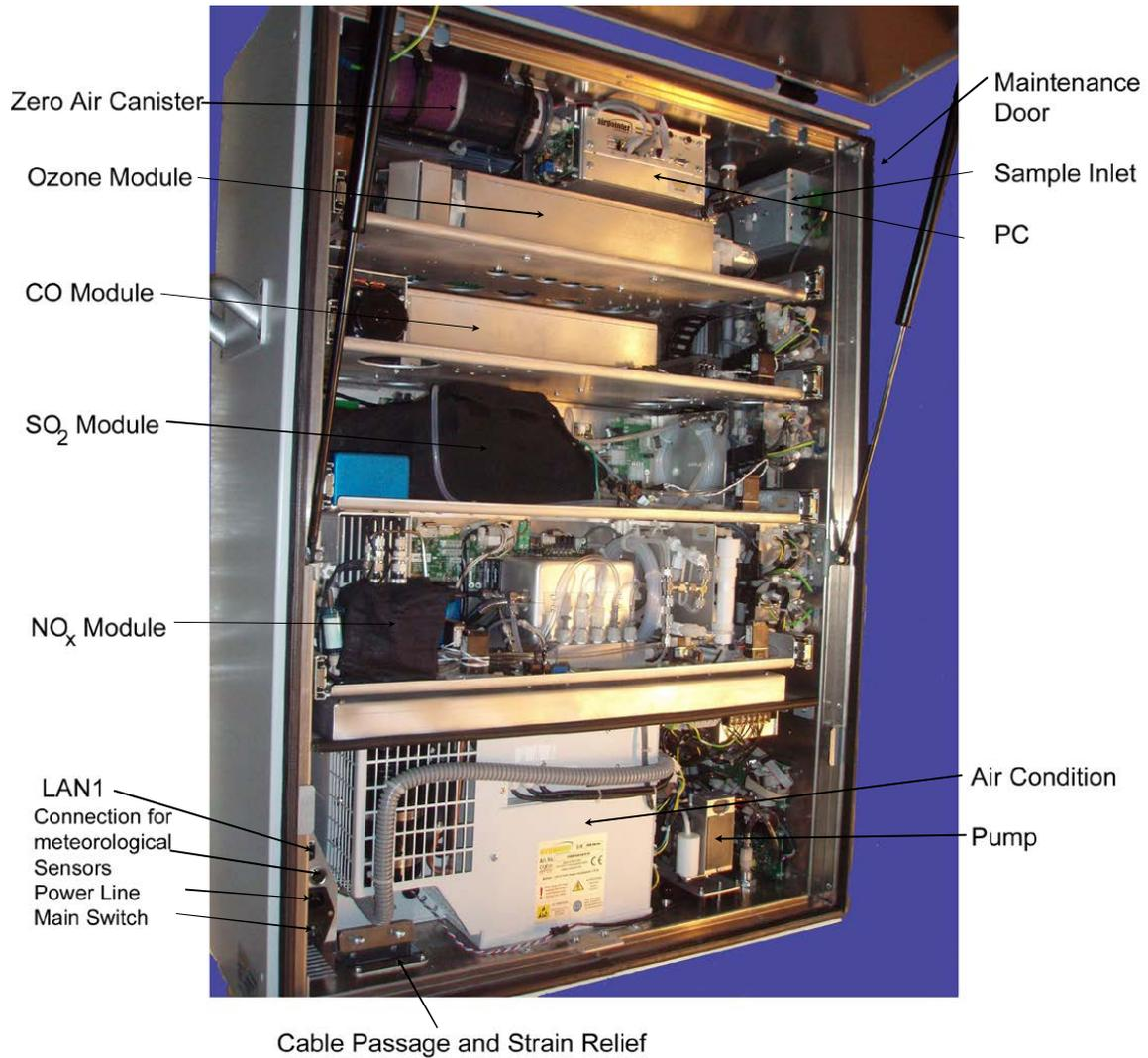
Figure 5.12.: Inside the airpointer® with four drawers (4D)
