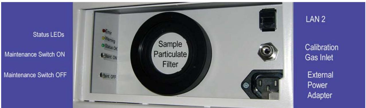
Figure 5.13.: Inside the Maintenance Door of the airpointer®
