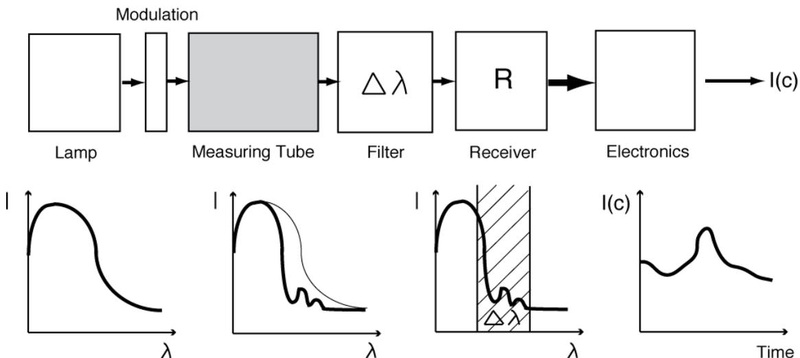
Figure 9.4.: Principle of Optical Light Detection
