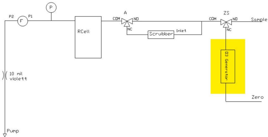
Figure 12.9.: Flow diagram of the ozone module with Internal Span Module
