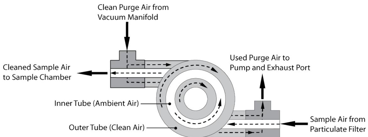
Figure 10.39.: Hydrocarbon Scrubber Scheme
