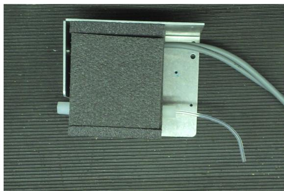
Figure 12.19.: Removed Internal Span Module with thermal insulation
