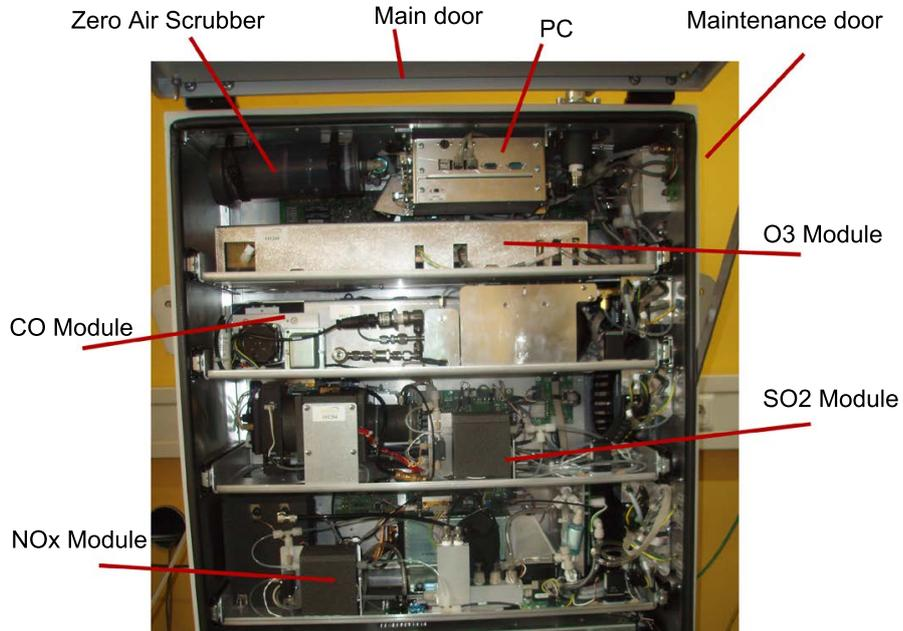
Figure 11.1.: Inside the airpointer® with four slides (4D) top
