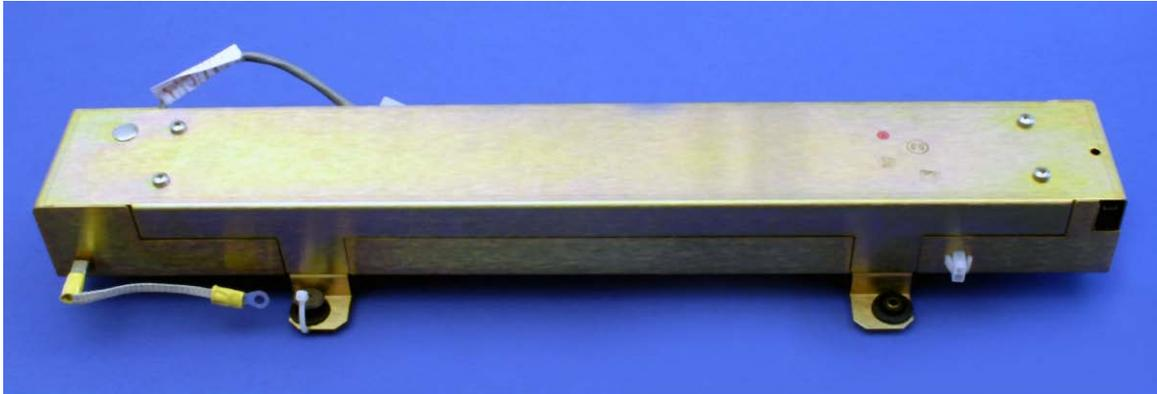
Figure 11.23.: Ozone Bench without Thermal Insulation
