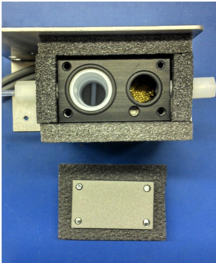
Figure 12.20.: Internal Span Module with unscrewed top and thermal insulation
