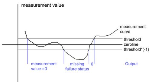
Figure 13.14.: Measurement Curve with Threshold
