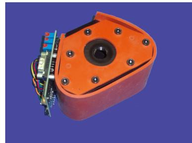
Figure 14.10.: Exterior View of a Nephelometer
