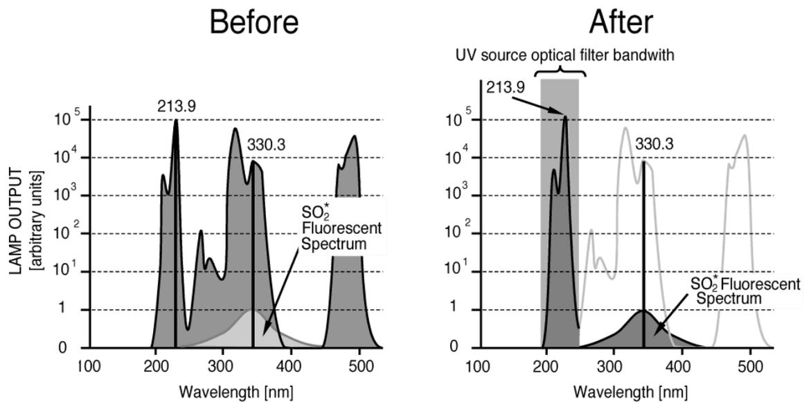
Figure 10.19.: Excitation Lamp UV Spectrum Before/After Filtration
