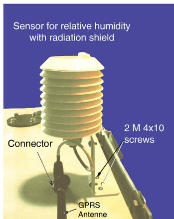
Figure 13.27.: Side View of the mounted sensor
