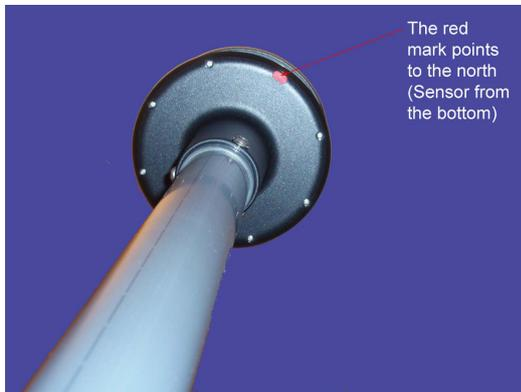
Figure 13.8.: North mark on the Gill sensor: The red point on the bottom side points north
