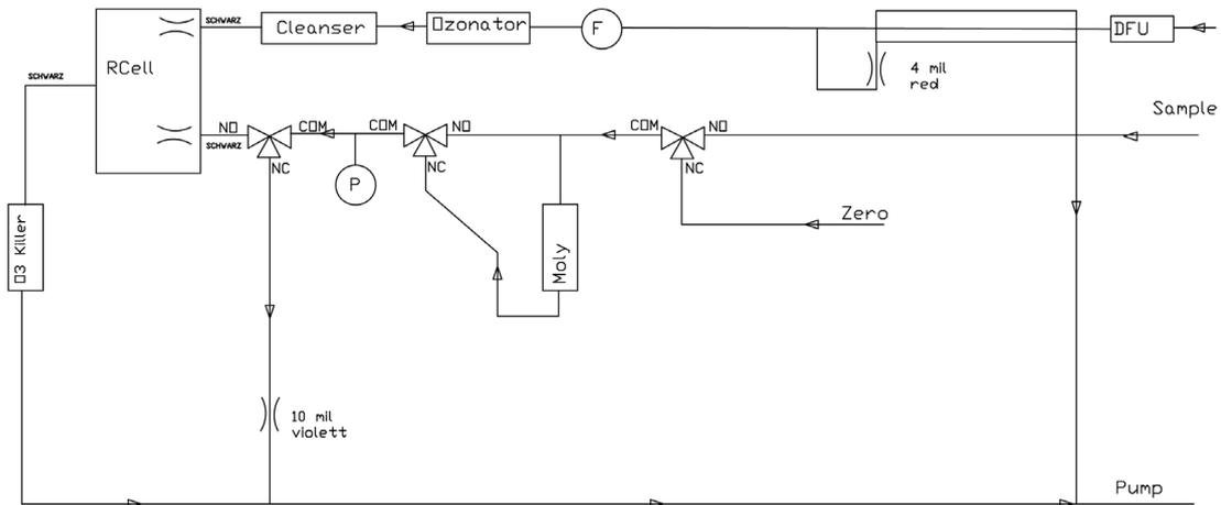
Figure 10.8.: Flow Diagram of NO<sub>x</sub> Module
