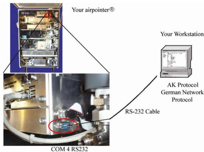
Figure A.1.: COM Port For Communication via AK and German Ambient Network Protocol
