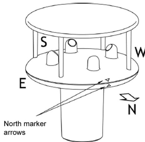
Figure 13.18.: Gill Sensor with Compass Points
