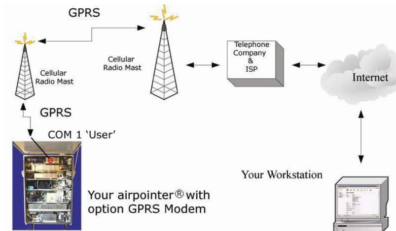
Figure 6.3.: GPRS Connection
