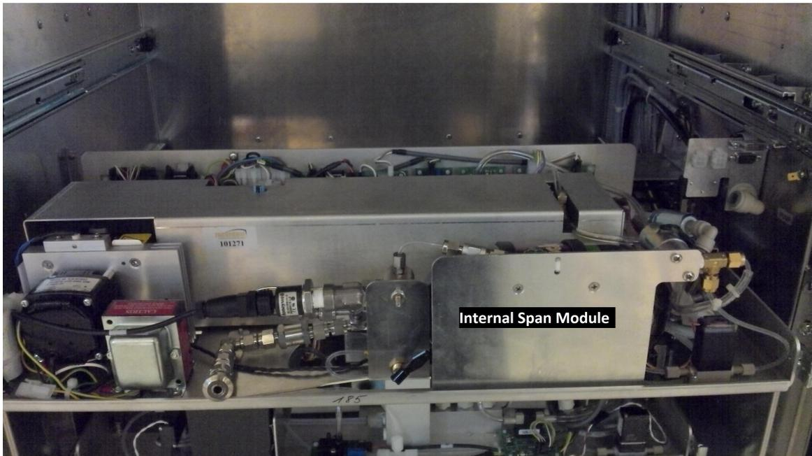
Figure 12.14.: Location of the Internal Span Module on the CO module
