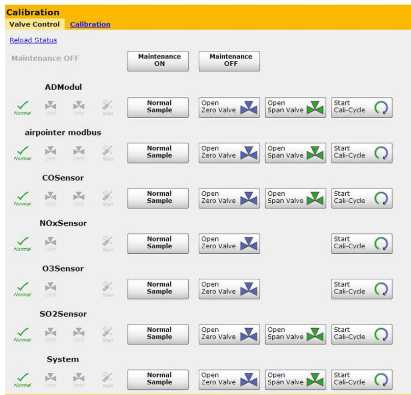
Figure 7.17.: Deactivate the Maintenance Mode
