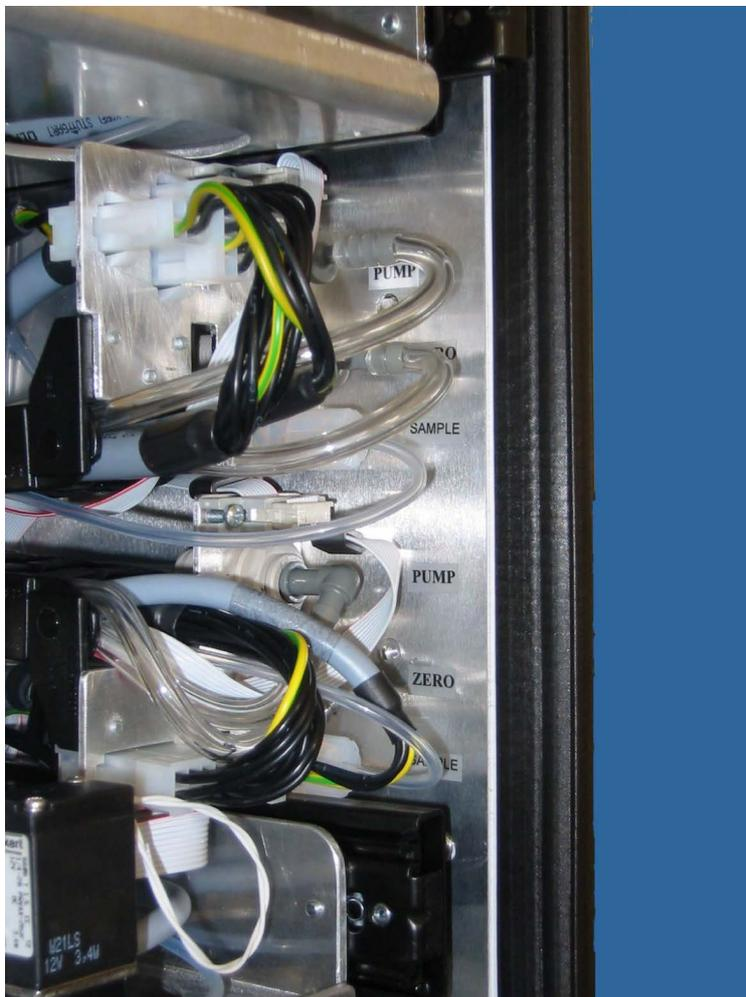
Figure 11.46.: Connection of the Flow Channel of a Module to the airpointer®
