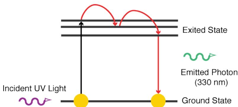
Figure 9.3.: An Excited Molecule Emits its Energy as a Light Pulse – Fluorescence.
