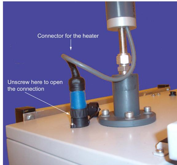
Figure 14.3.: Connect and Disconnect the Plug
