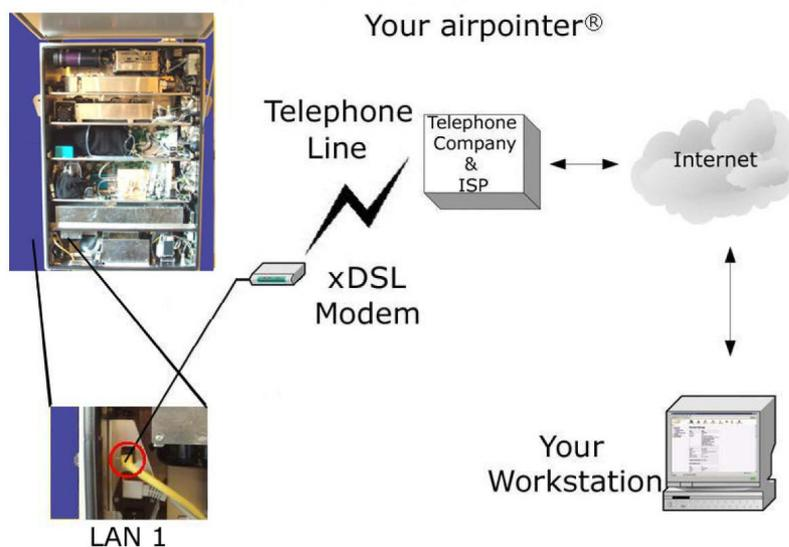
Figure 6.9.: ADSL and SDSL Connection
