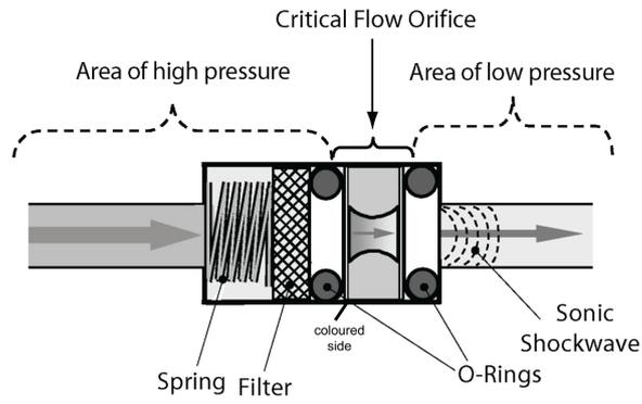
Figure 11.43.: Critical Flow Orifice of the NO Reaction Cell Scheme
