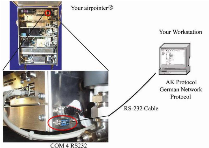
Figure 6.10.: Connection Using AK or German Ambient Network Protocol
