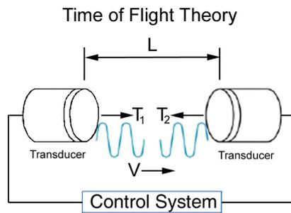
Figure 13.19.: Gill Sensor - Principle of Operation
