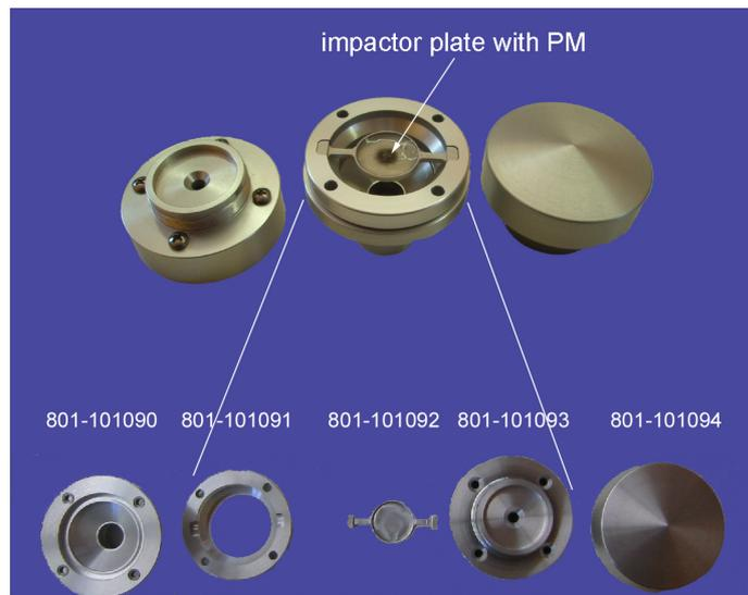
Figure 14.17.: PM10 Head Disassembled
