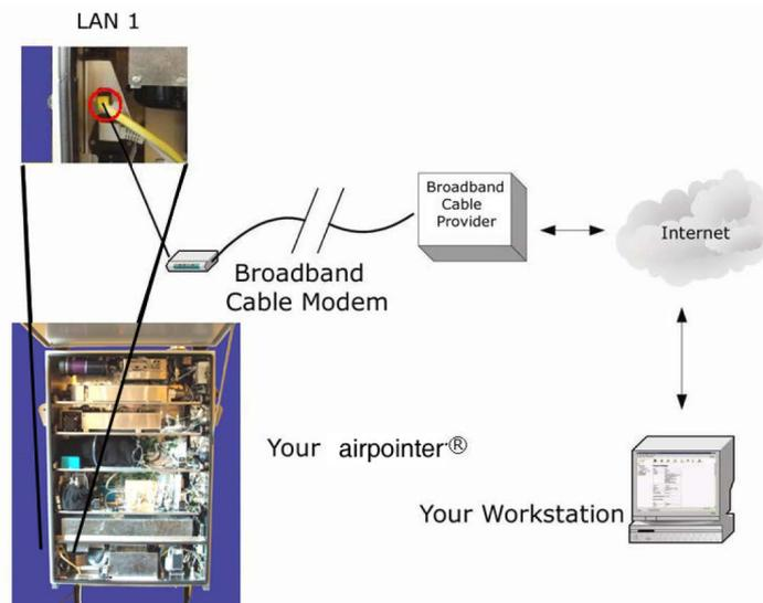
Figure 6.8.: Cable Modem Connection
