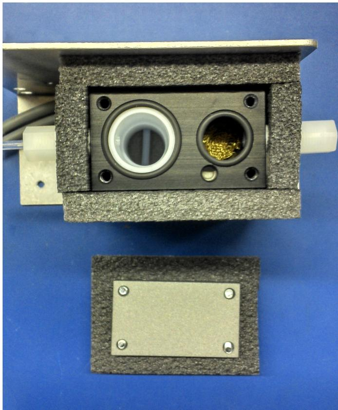
Figure 12.25.: Internal Span Module with unscrewed top and thermal insulation
