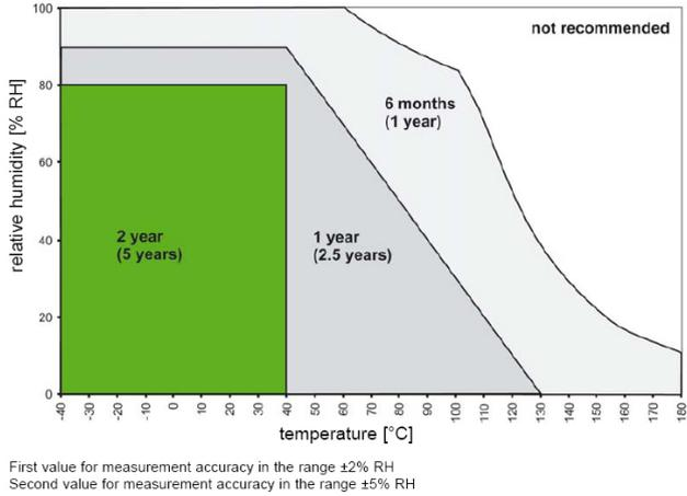
Figure 13.33.: Recalibration Interval for Humidity Sensor
