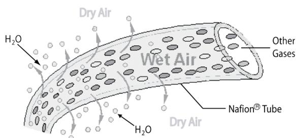
Figure 10.13.: Semi-Permeable Membrane Drying Process
