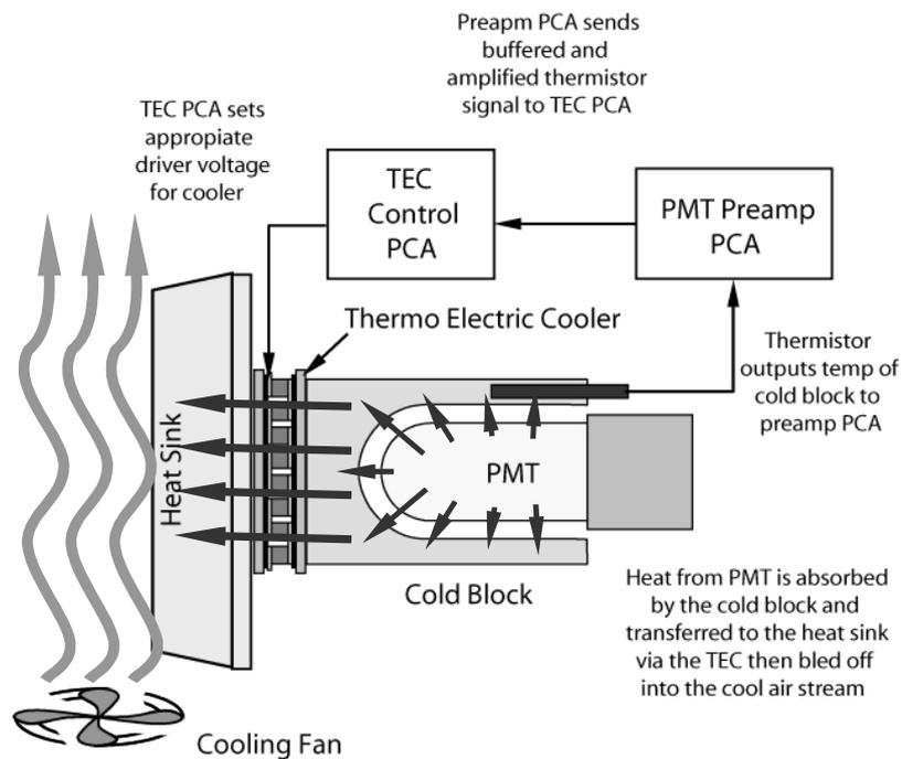
Figure 10.38.: PMT Cooling System
