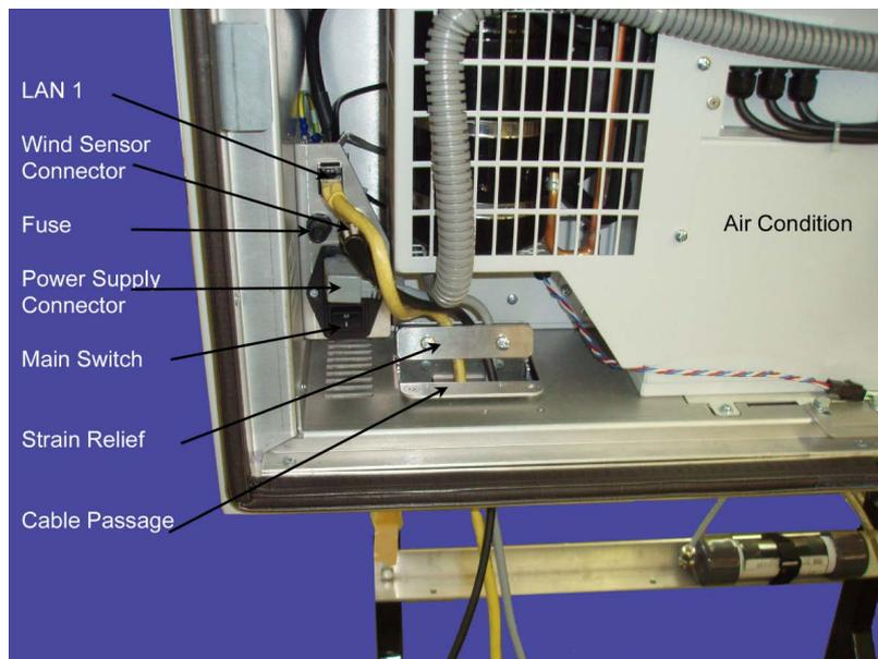
Figure 5.19.: Position of the Power Supply and Connector of the Master Switch, at the Left Bottom of the airpointer®
