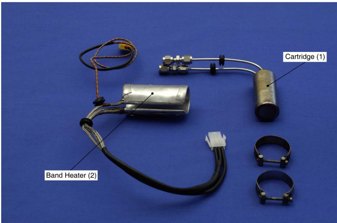
Figure 11.36.: Cartridge and Band Heater
