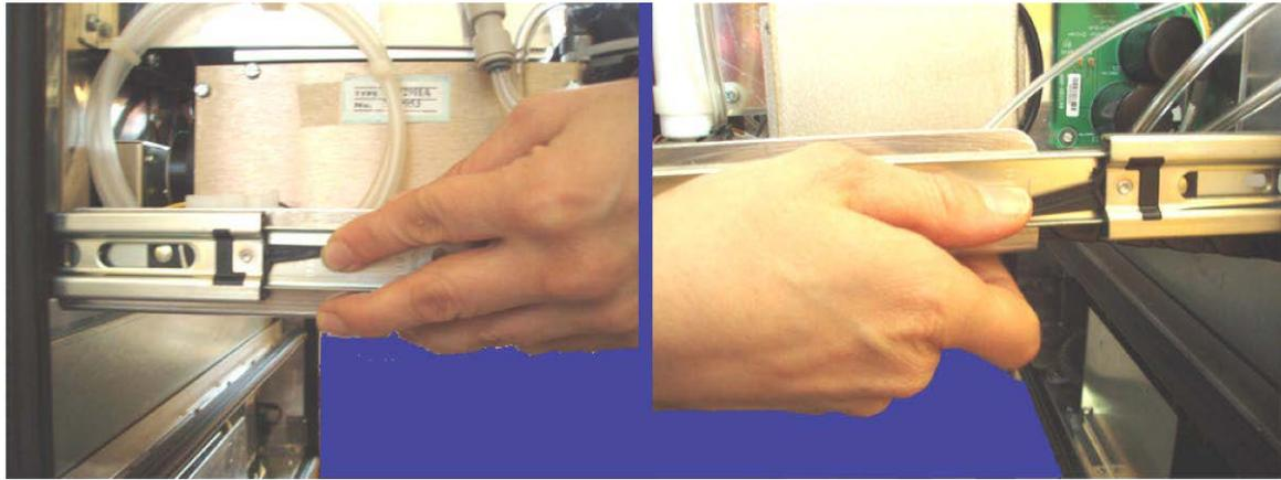
Figure 11.11.: Press the small levers in both drawers up (left) or down (right).
