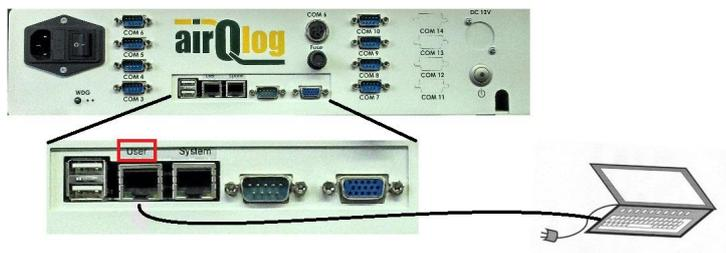
Figure 5.9.: direct connection with the cross patch cable
