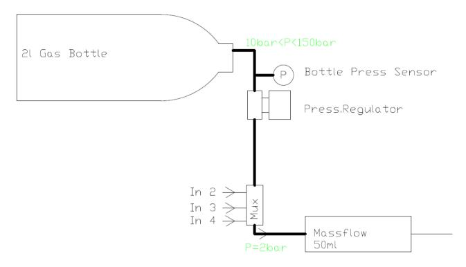
Figure 7: Pneumatic diagram of the high-pressure tubing of the mobile airQrate
