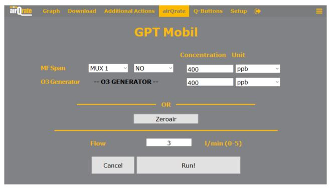
Figure 19: generating NO2 using the GPT module
