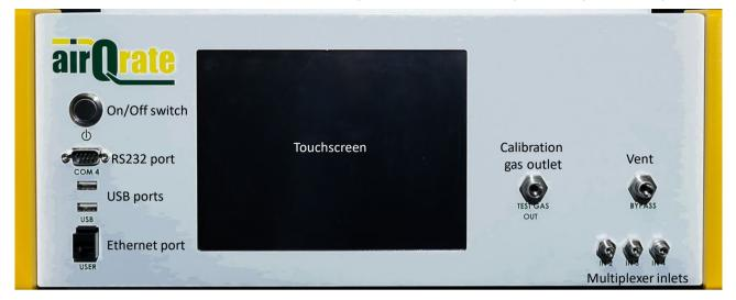
Figure 2: Front view of the mobile airQrate
