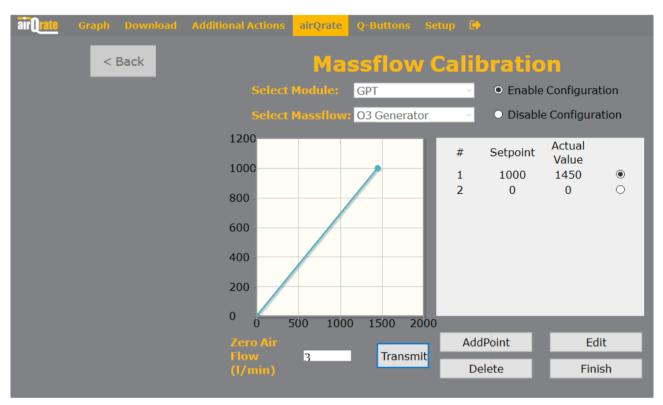
Figure 38: Recalibrating the ozone generator
