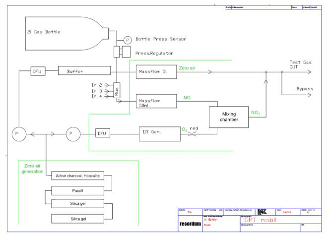
Figure 1: Pneumatic diagram of the AirQrate GPT mobile
