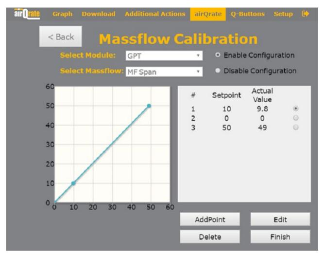
Figure 37: Calibration curve of the MF displayed as a graph and as numerical values
