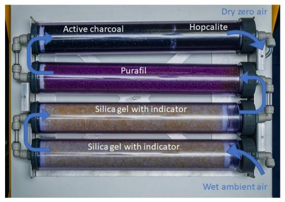
Figure 41: Cartridges generating zero air
