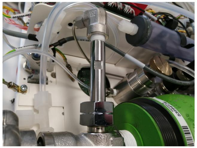
*Figure 5: Connecting the internal cylinder*
