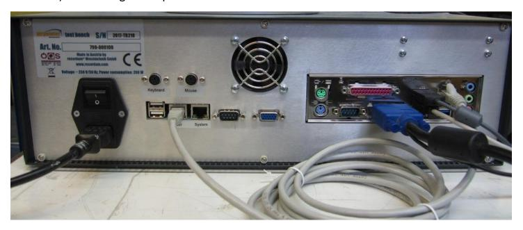
Connect workstation PC and airpointer PC "User interface" via network cable.
