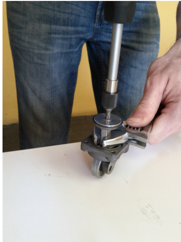
Figure 3.14: Fasten the screw of the con rod
