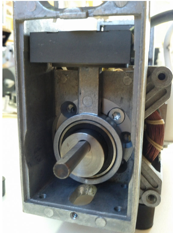
Figure 3.18: Flattening of the shaft must point up
