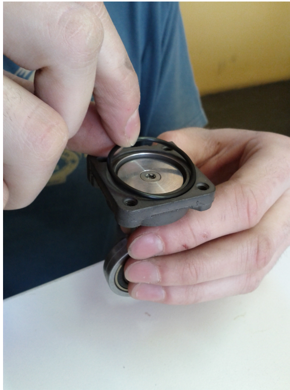
Figure 3.15: Put on the second sealing ring
