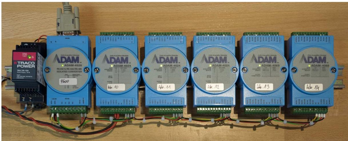
NOTE: There is a little switch on the side of the module, this need to be in the “Normal” position to work correct! (In the Init position it is answering only to Address 0)
